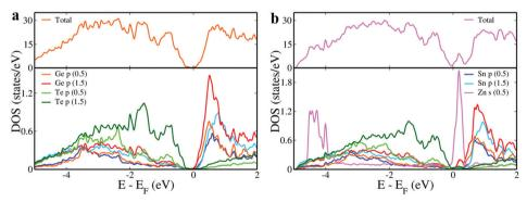
Fig. 2 pDOS of (a) Sn<sub>10</sub>Ge<sub>6</sub>Te<sub>16</sub> and (b) Sn<sub>9</sub>Ge<sub>6</sub>ZnTe<sub>16</sub>. The energy levels are shifted with respect to the Fermi level of the configurations, which is set to
