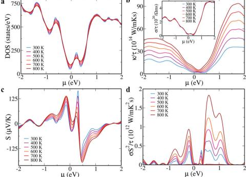
Fig. 3 (a) DOS, (b) thermal conductivity (inset: electrical conductivity), (c) Seebeck co-efficient and (d) power factor of  $Sn_9Ge_6ZnTe_{16}$  as a function of chemical potential ( $\mu$ ) at various temperatures. The conductivity and power factor values are reported by scaling them with  $\tau$ .
