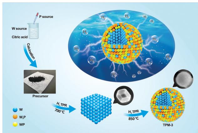
Fig. 1 Schematic illustration of the synthesis procedure.
