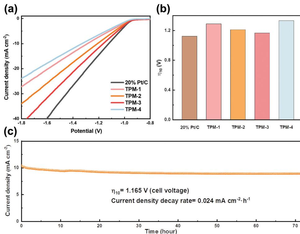
Fig. 7 Electrocatalytic HER performance of TPM-1, TPM-2, TPM-3, TPM-4, and 20 wt% Pt/C in simulated seawater (1 M KOH, 0.5 M NaCl,  $41.2 \times 10^{-3} \text{ M}$  MgCl<sub>2</sub> and  $12.5 \times 10^{-3} \text{ M}$  CaCl<sub>2</sub>). (a) Polarization curves, (b) overpotentials of Pt/C and TPMs for achieving a current density of  $10 \text{ mA cm}^{-2}$ , and (c) the  $i-t$  curve at a cell voltage of 1.165 V for TPM-3.
