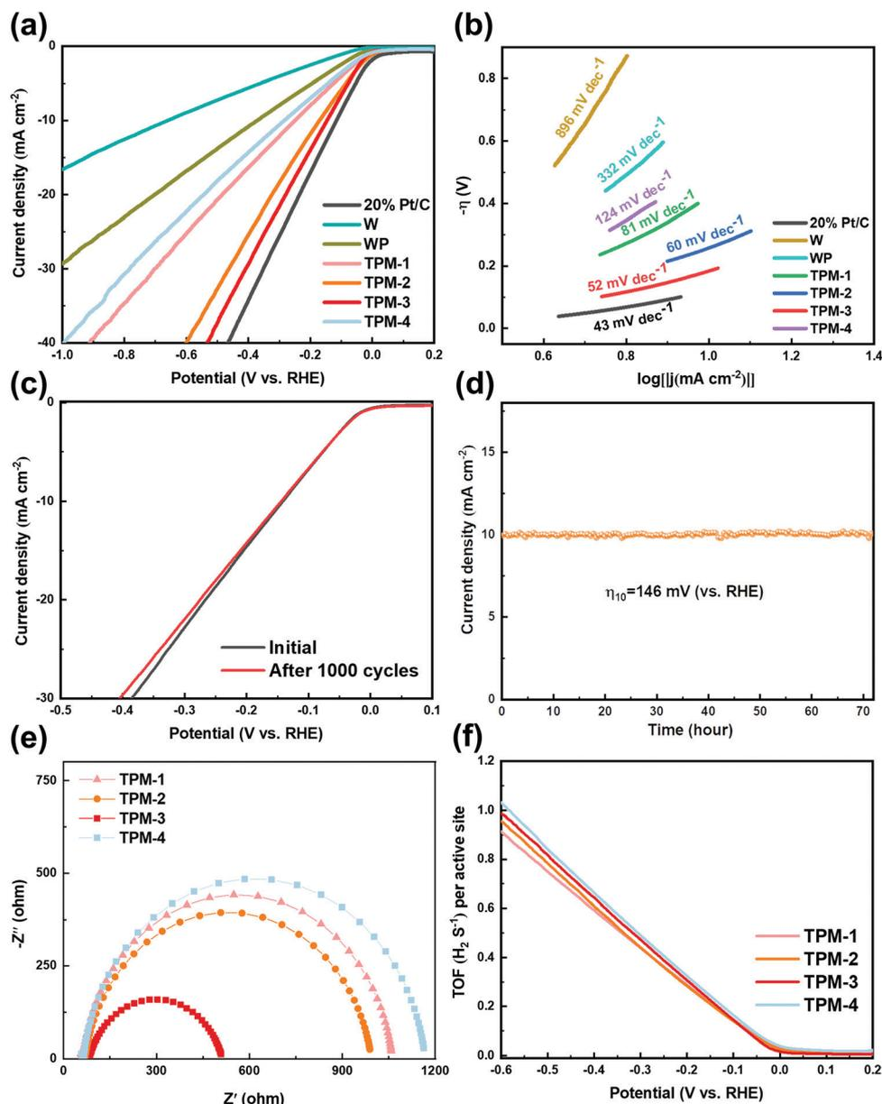
Fig. 6 Electrocatalytic HER performance of TPM-1, TPM-2, TPM-3, TPM-4, W, WP, as well as 20 wt% Pt/C in alkaline (1 M KOH) media. (a) Polarization curves, (b) corresponding Tafel slope diagrams, (c) LSV curves before and after 1000 CV cycles for TPM-3, (d)  $i-t$  curve at overpotential of 146 mV for TPM-3, (e) EIS curves and (f) TOF profiles of TPMs.
