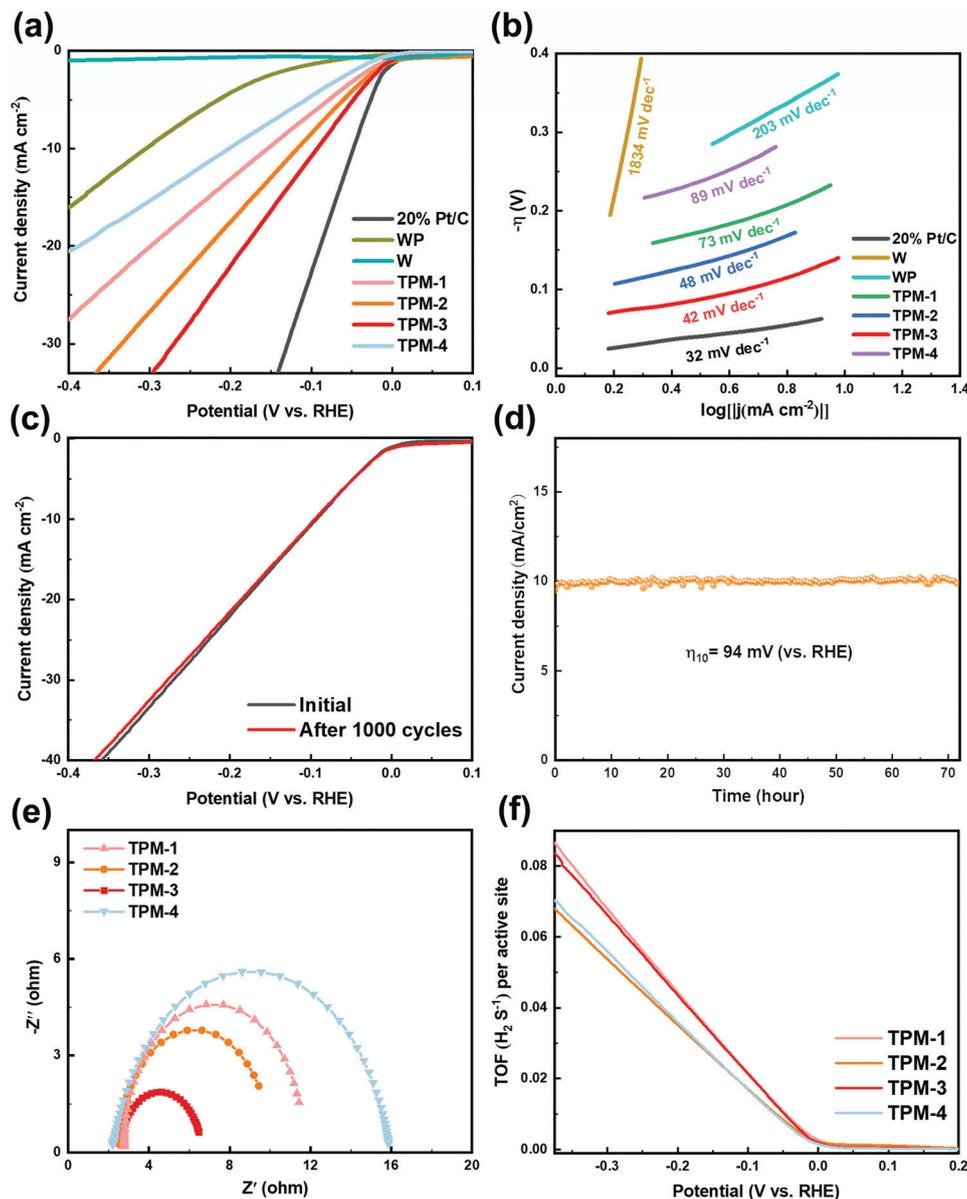
Fig. 5 The electrocatalytic HER performance of TPM-1, TPM-2, TPM-3, TPM-4, W, WP, as well as 20 wt% Pt/C in acid (0.5 M  $\text{H}_2\text{SO}_4$ ) media. (a) Polarization curves; (b) corresponding Tafel slope diagrams; (c) LSV curves before and after 1000 CV cycles for TPM-3; (d)  $i-t$  curve at an overpotential of 94 mV for TPM-3; (e) EIS curves and (f) TOF profiles of the TPMs.
