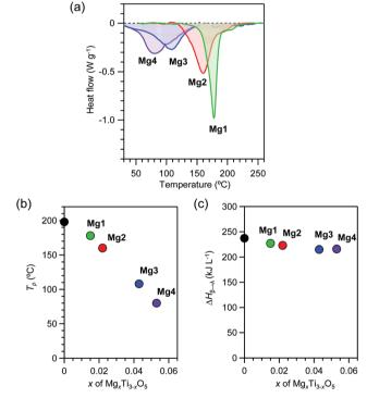
Fig. 4 Heat-storage properties of  $\lambda$ -Mg<sub>x</sub>Ti<sub>3-x</sub>O<sub>5</sub>. (a) DSC charts of **Mg1** (green), Mg2 (red), Mg3 (blue), and Mg4 (purple) as the temperature increases. (b) x-Value dependence of the transition temperature. (c) x-Value dependence of the transition enthalpy. Black circle represents block-type  $\lambda$ -Ti<sub>3</sub>O<sub>5</sub> (adapted from ref. 15).
