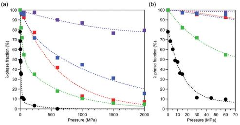
Fig. 2 (a) Pressure dependence of the  $\lambda$ -phase fractions of  $\lambda$ -Mg<sub>x</sub>Ti<sub>3-x</sub>O<sub>5</sub> for **Mg1** (green), **Mg2** (red), **Mg3** (blue), **Mg4** (purple), and block-type  $\lambda$ -Ti<sub>3</sub>O<sub>5</sub> (black, adapted from ref. 15). (b) Enlarged plot in the low pressure region. Dashed lines are to guide the eye.
