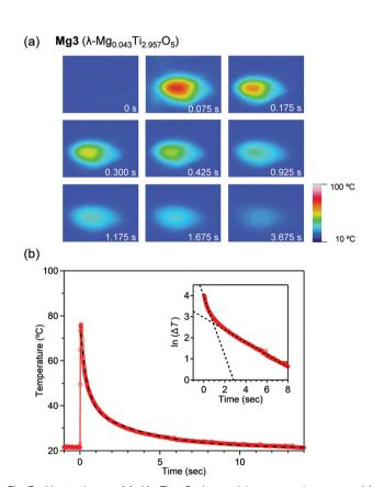
Fig. 3 Heat release of  $\lambda$ -Mg<sub>x</sub>Ti<sub>3-x</sub>O<sub>5</sub> by applying external pressure. (a) Thermographs for Mg3. Color scale of the temperature is shown on the right. (b) Decay of the maximum temperature within a square area after applying pressure to Mg3 at t = 0.
