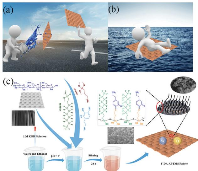
Fig. 1 The F-DA-APTMS fabric is expected to be endowed with (a) excellent anti-fouling and (b) high buoyancy. (c) Preparation of a robust F-DA-APTMS superamphiphobic fabric by an *in situ* one-pot method.
