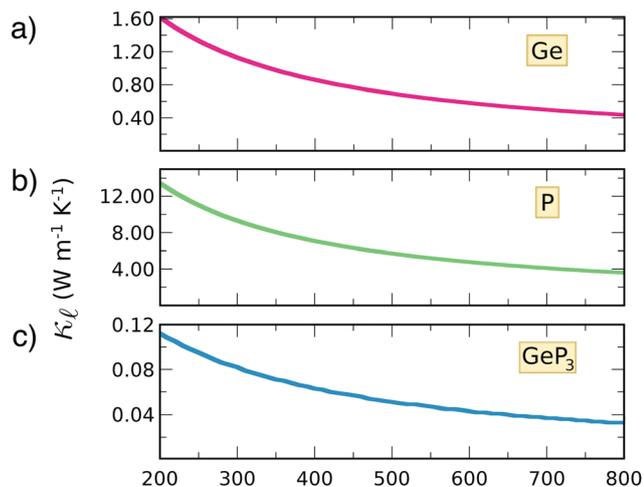
Fig. 6 Thermal conductivity as a function of temperature for (a) germanene; (b) blue P and (c) GeP<sub>3</sub>.
