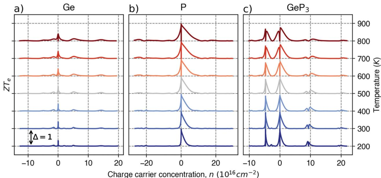
Fig. 4 The electronic figure of merit at different temperatures for: (a) germanene, (b) blue P and (c) GeP<sub>3</sub>.
