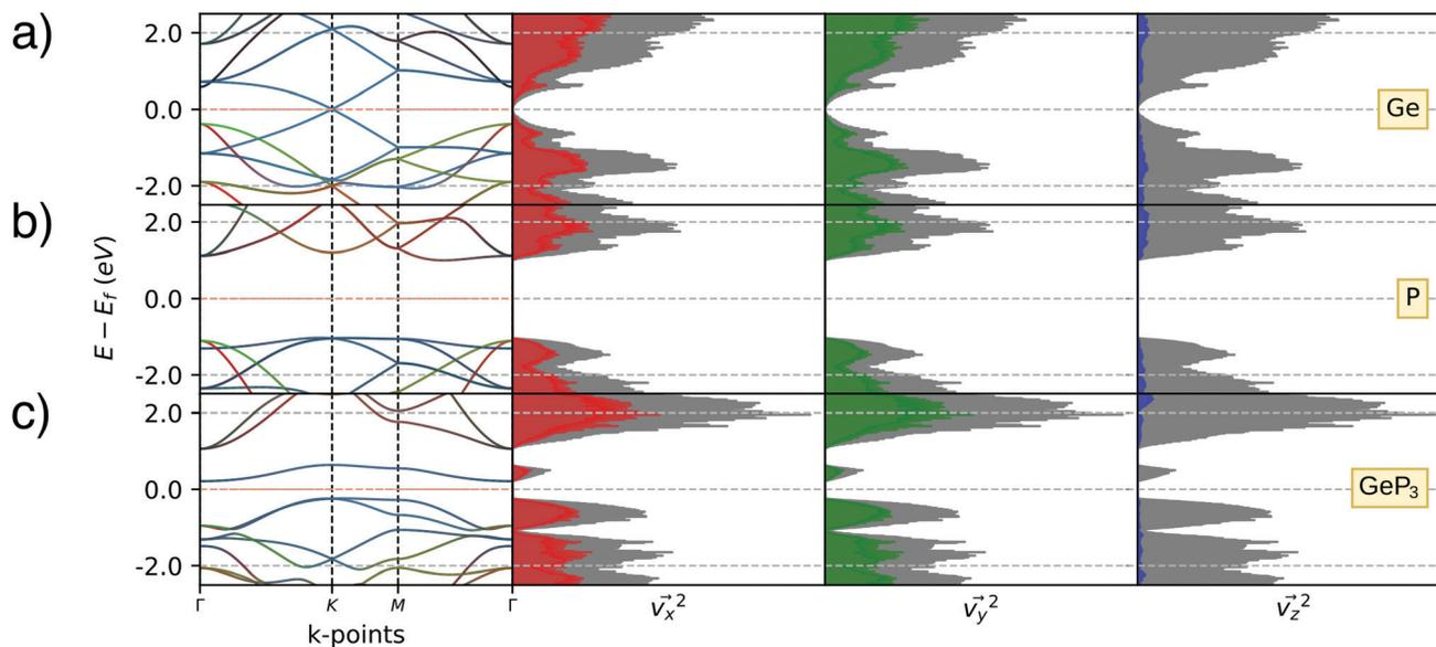
Fig. 2 Band structure projected over p orbitals for (a) Ge; (b) blue P; (c) GeP<sub>3</sub>, with the respective squares of group velocity components on the right panels. Red, green, blue and light gray represent  $v_x^2$ ,  $v_y^2$ ,  $v_z^2$  and total  $v^2$ , respectively. The Fermi level,  $E_f$ , is set to zero. The colors red, green and blue also represents the orbitals  $p_x$ ,  $p_y$  and  $p_z$ , respectively.
