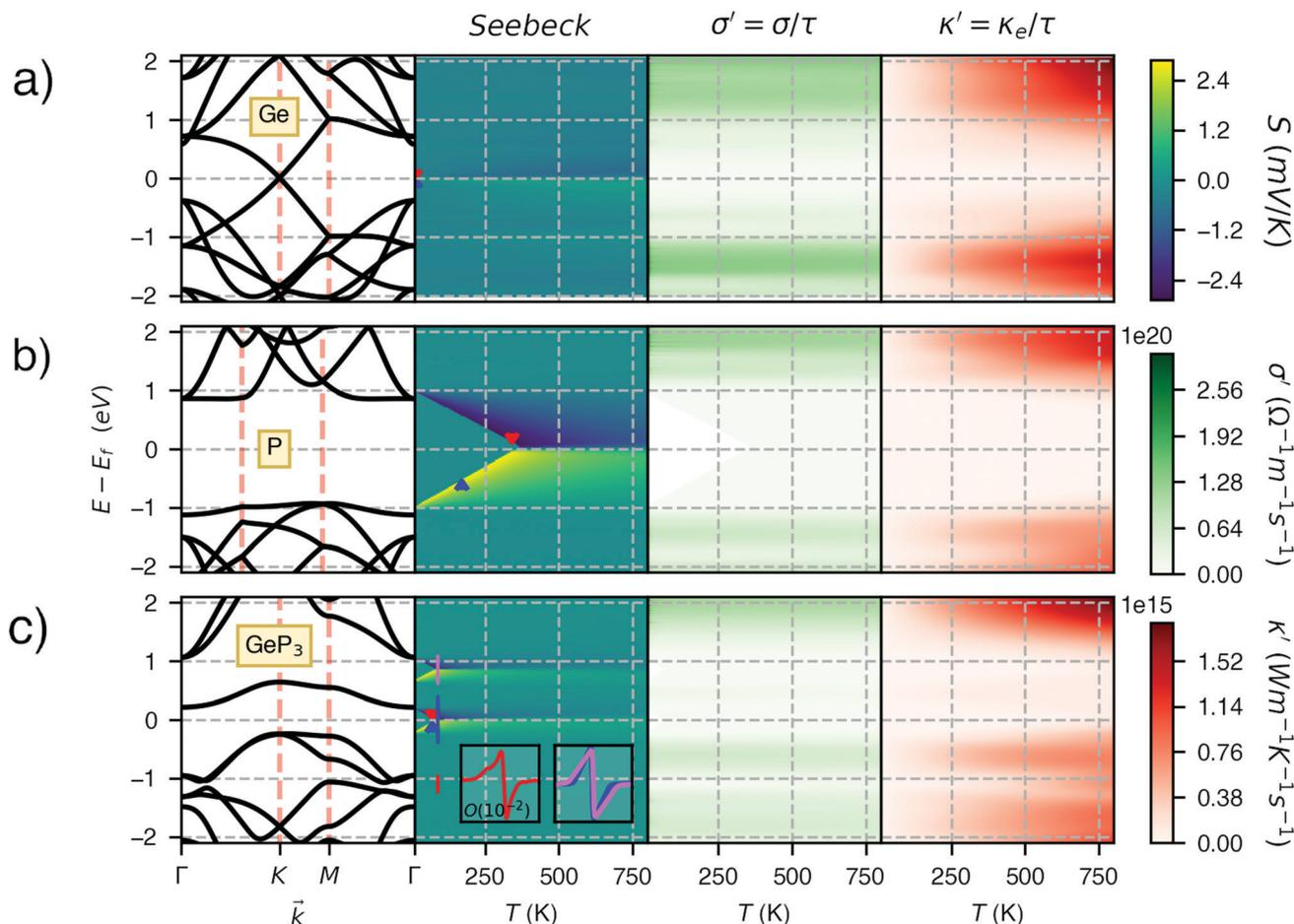
Fig. 3 The band structure  $E(k)$ , the Seebeck coefficient  $S$ , scaled electrical conductivity  $\sigma' = \sigma/\tau$  and electronic thermal conductivity  $\kappa'_e = \kappa_e/\tau$  for (a) Ge, (b) blue P and (c)  $\text{GeP}_3$ . The Fermi level is set at zero. The red and blue arrows indicate the location of the maximum and minimum values, respectively, of  $S$  for each material.
