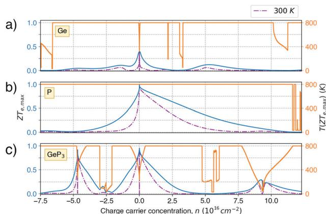
Fig. 5 Maximum value of  $ZT_e$  ( $ZT_{e,max}$ , full blue line) and the temperature at which it occurs ( $T(ZT_{e,max})$ , orange full line) as a function of charge carrier concentration  $n$  for the three materials studied for (a) germanene; (b) blue P and (c) GeP<sub>3</sub>.  $ZT_e$  ( $T = 300$  K) curves are also presented in dash-dotted purple lines.
