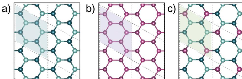
Fig. 1 Top views of fully relaxed atomic structures for (a) Ge, (b) blue P and (c)  $\text{GeP}_3$ . The shadowed regions depict the unit cell for  $\text{GeP}_3$ , and supercells for Ge and blue P. Darker and lighter atom shades indicate lower and higher vertical position regarding buckling planes, respectively.
