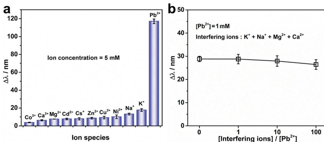
Fig. 5 Selectivity of the PNBC hydrogel sensor toward  $Pb^{2+}$ . (a) Effect of ion species on  $\Delta\lambda$  in aqueous solutions containing each ion at a concentration of 5 mM at 25 °C. (b) Effect of interfering ions on  $\Delta\lambda$  in a 1 mM  $Pb^{2+}$  solution containing various interfering ions ( $K^+$ ,  $Na^+$ ,  $Mg^{2+}$  and  $Ca^{2+}$ ) in which the concentration of the interfering ions is changed from 1 to 100 mM.
