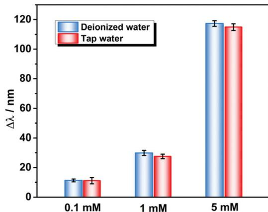
Fig. 6 Detection performance of the PNBC hydrogel sensor toward  $\text{Pb}^{2+}$  at various concentrations in DI water and tap water.
