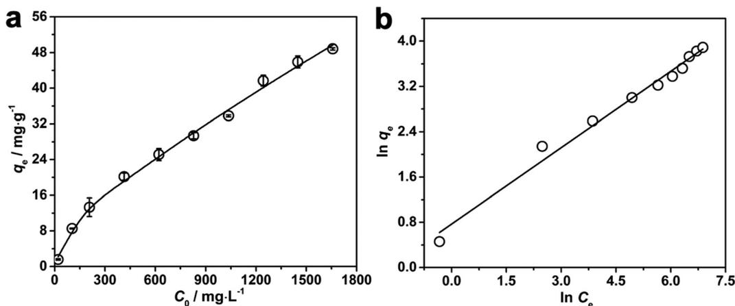
Fig. 8 (a) Adsorption performance of the PNBC photonic hydrogel sensor toward  $\text{Pb}^{2+}$  in water, where the  $\text{Pb}^{2+}$  concentration is varied from 0 to  $1650 \text{ mg L}^{-1}$ , and (b) fitting curve of the Freundlich isotherm model for  $\text{Pb}^{2+}$  adsorption onto the PNBC photonic hydrogel. The use of the hydrogel is  $14 \text{ g L}^{-1}$ , the operating temperature is  $25 \text{ }^\circ\text{C}$ , and the pH value is 5.5.
