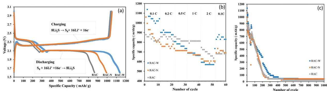
Fig. 5 (a) Galvanostatic charge/discharge profiles at 0.1C rate, (b) C-rate test, (c) Stability test of LSBs using RAC, RAC-W and RAC-N as active materials.
