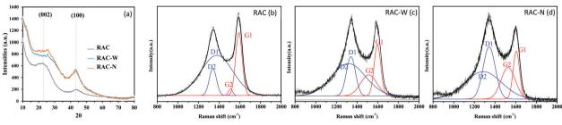
Fig. 3 (a) XRD patterns of RAC, RAC-W and RAC-N as well as Raman spectra of (b) RAC, (c) RAC-W, and (d) RAC-N.
