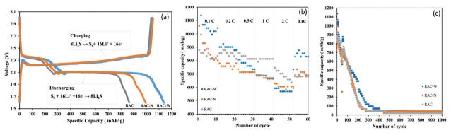
Fig. 5 (a) Galvanostatic charge/discharge profiles at 0.1C rate, (b) C-rate test, (c) Stability test of LSBs using RAC, RAC-W and RAC-N as active materials.
