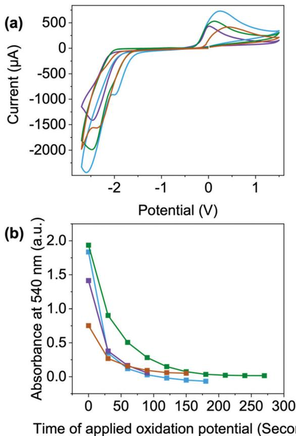
Fig. 7 (a) Cyclic voltammograms collected from buffered 10 mg mL<sup>-1</sup> solutions of **NDI-I** (—), **NDI-V** (—) adjusted to pH 9 and **NDI-F** (—) and **NDI-GF** (—) adjusted to pH 6 voltammograms measured in 1 × 1 cm FTO windows. The scan rate of the cyclic voltammograms was 0.1 V s<sup>-1</sup>. (b) Time taken after the application of the oxidising potential for the absorbance at 540 nm to return to 0.
