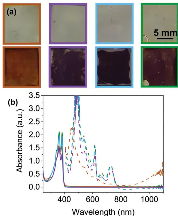
Fig. 6 (a) Photographs of **NDI-I** (—), **NDI-V** (—) adjusted to pH 9 and **NDI-F** (—) and **NDI-GF** (—) adjusted to pH 6 in their neutral (top) and reduced states (bottom) (b) absorbance spectra of same solutions in neutral (solid line) and reduced (dashed line) state. Because of absorbance from FTO glass over 400 nm, this section of the data is removed. Intensity of absorbance at 485 nm is too large for the spectrometer.
