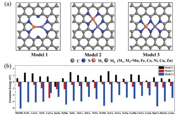
Fig. 1 (a) Geometric structures and (b) formation energies of  $M_1/M_2-N_6-Gra$  ( $M_1/M_2=Mn-Zn$ ). The gray, blue, orange, and purple atoms represent carbon, nitrogen,  $M_1$ , and  $M_2$ , respectively.
