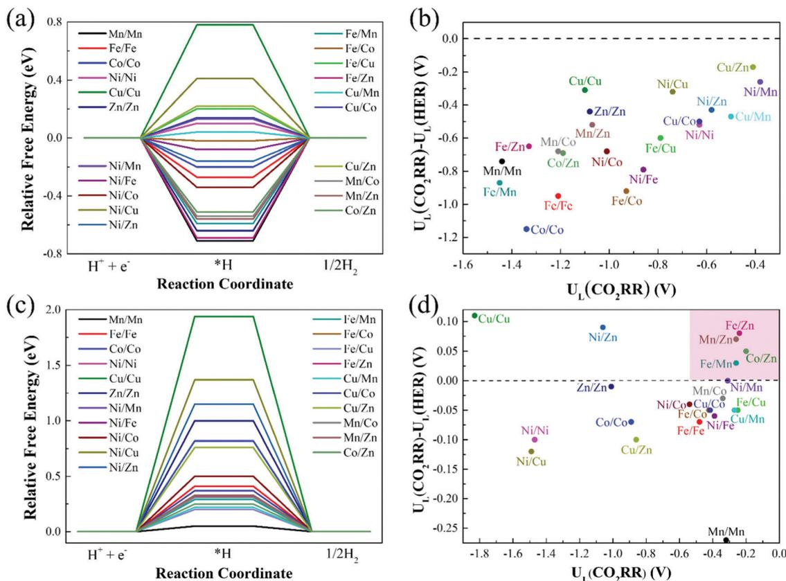
Fig. 7 Relative free energy profiles for HER on (a) Model 2 and (c) Model 3, and limiting potential difference between CO<sub>2</sub>RR and HER for (b) Model 2 and (d) Model 3.
