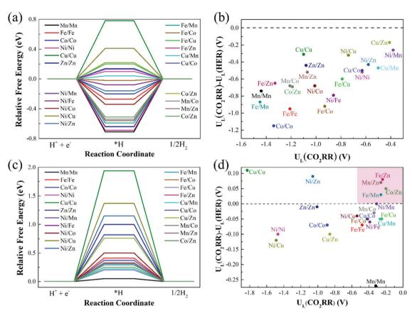
Fig. 7 Relative free energy profiles for HER on (a) Model 2 and (c) Model 3, and limiting potential difference between CO<sub>2</sub>RR and HER for (b) Model 2 and (d) Model 3.
