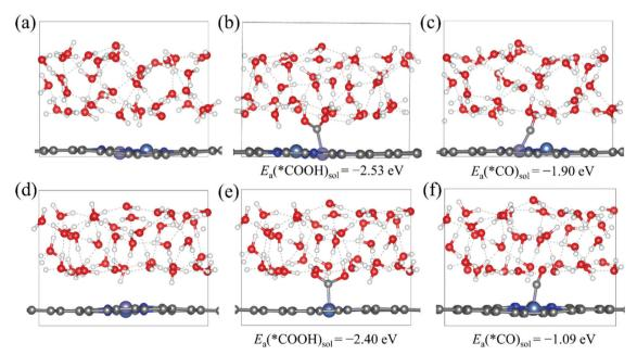
Fig. 3 The explicit solvent models of the NiFe-N<sub>6</sub>-Gra (a) Model 2 and (d) Model 3 surface, \*COOH and \*CO configurations and adsorption energies at (b) and (c) water/Model 2 interface and (e) and (f) water/Model 3 interface.
