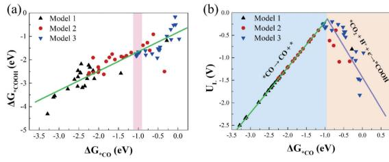
Fig. 6 (a) The scaling relations of the adsorption free energies of \*COOH ( $\Delta G_{*COOH}$ ) and \*CO ( $\Delta G_{*CO}$ ), (b) the volcano plot between the limiting potentials ( $U_{\rm L}$ ) and  $\Delta G_{^{\star}{\rm CO}}$
