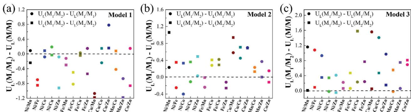
Fig. 5 (a)–(c) The limiting potential difference between heteronuclear  $M_1/M_2-N_6$ -Gra and homonuclear  $M/M-N_6$ -Gra ( $M_1/M_1-N_6$ -Gra,  $M_2/M_2-N_6$ -Gra) for Model 1, Model 2 and Model 3. ( $U_L(M_1/M_2) - U_L(M/M)$ ) > 0 means that the catalytic activity of heteronuclear  $M_1/M_2-N_6$ -Gra catalysts are higher than the homonuclear  $M/M-N_6$ -Gra.
