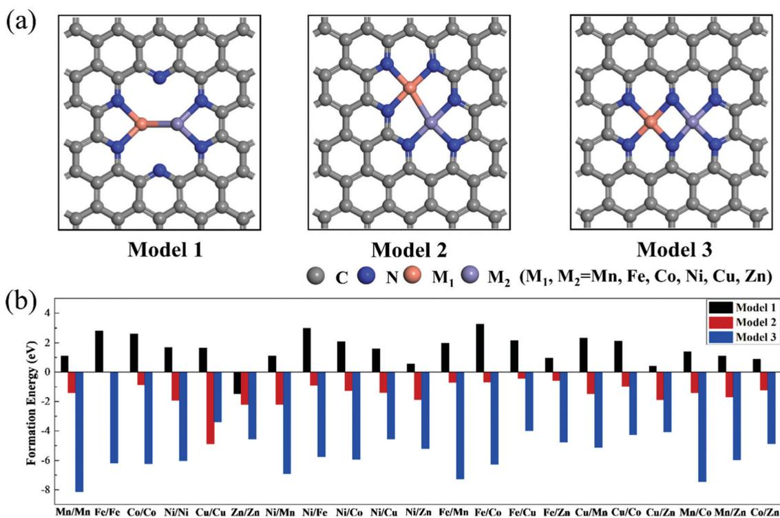
Fig. 1 (a) Geometric structures and (b) formation energies of  $M_1/M_2\text{-N}_6\text{-Gra}$  ( $M_1/M_2 = \text{Mn-Zn}$ ). The gray, blue, orange, and purple atoms represent carbon, nitrogen,  $M_1$ , and  $M_2$ , respectively.
