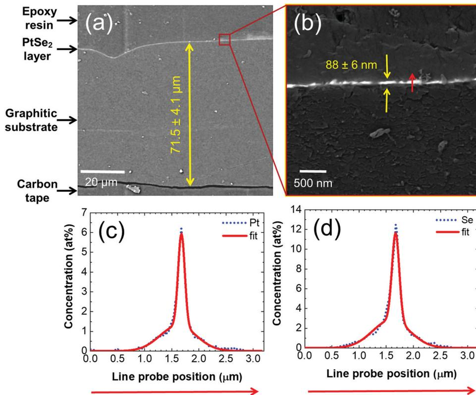
Fig. 2 (a) Polished cross-section SEM image of the material revealing both the thickness of the PtSe<sub>2</sub> film and the rGO substrate. (b) Detailed microstructure of the PtSe<sub>2</sub>/rGO foil showing the thickness of the PtSe<sub>2</sub> film. The red arrow denotes an EDS elemental line probe for (c) Pt and (d) Se elements.
