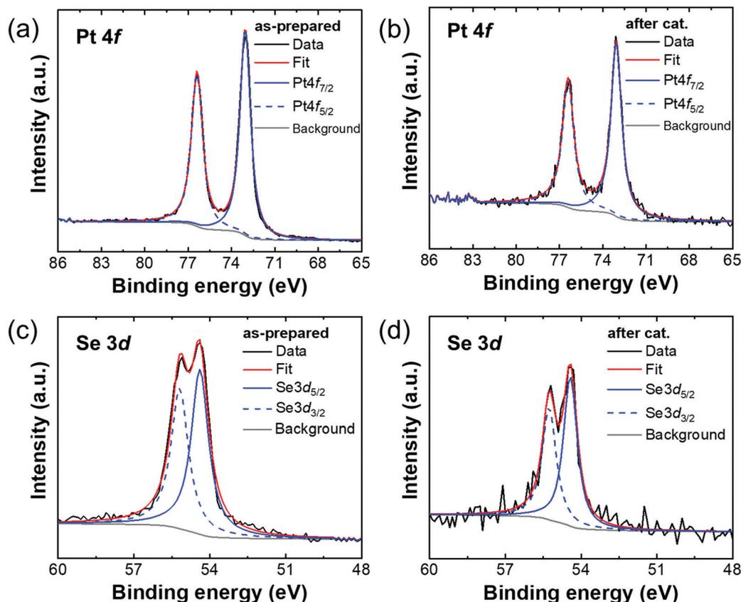
Fig. 7 XPS spectra of core levels: (a and b) Pt 4f and (c and d) Se 3d with respective deconvolution of peaks and assignment of components for the PtSe<sub>2</sub> foil on the PtSe<sub>2</sub> side. Left- and right-hand spectra are for as-prepared samples and samples after long-term stability tests, respectively.
