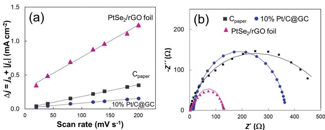
Fig. 4 (a) Plots of the capacitive current density at 1.1 V vs. RHE for the determination of  $C_{dl}$  and (b) the respective Nyquist plot for the determination of  $R_{ct}$  of materials at  $-0.05 \text{ V vs. RHE}$ . The fitting of the Nyquist experimental curves is shown as a continuous line. Tested materials: C<sub>paper</sub>, 10% Pt/C@GC, and PtSe<sub>2</sub>/rGO foil.
