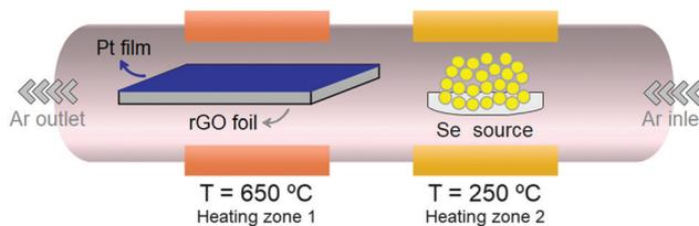
Scheme 1 Illustration of the PtSe<sub>2</sub> synthesis on an rGO foil.
