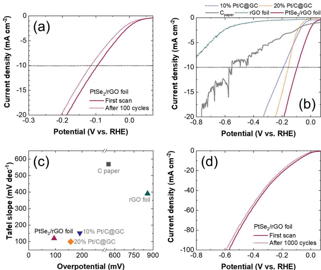
Fig. 3 HER performance in 1.0 M KOH. (a) LSV polarization curves of PtSe<sub>2</sub>/rGO foil. (b) Comparison of PtSe<sub>2</sub>/rGO foil LSV polarization curves with those of other catalysts and (c) the corresponding correlation between Tafel slope and overpotential at  $-10 \text{ mA cm}^{-2}$ . (d) Polarization curves of the PtSe<sub>2</sub>/rGO foil before and after 1000 cycles. Scan rate:  $2 \text{ mV s}^{-1}$ .
