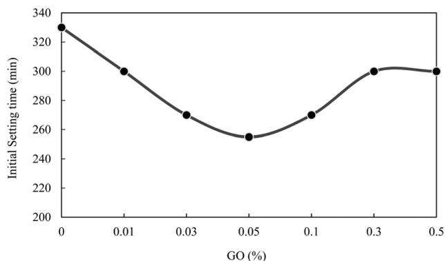
Fig. 2 Initial setting time of cement mortars.
