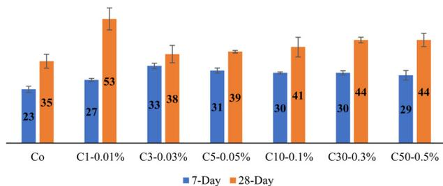
Fig. 6 Compressive strength (MPa) of GO-incorporated cement mortars.
