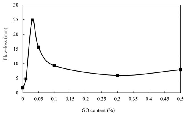
Fig. 4 Changes in flow-loss vs. GO content.
