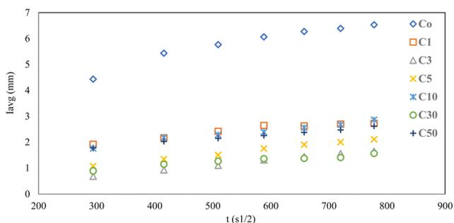
Fig. 11 Secondary water absorption rate of specimens.
