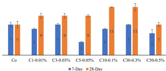
Fig. 7 Flexural strength (MPa) of GO-incorporated cement mortars.
