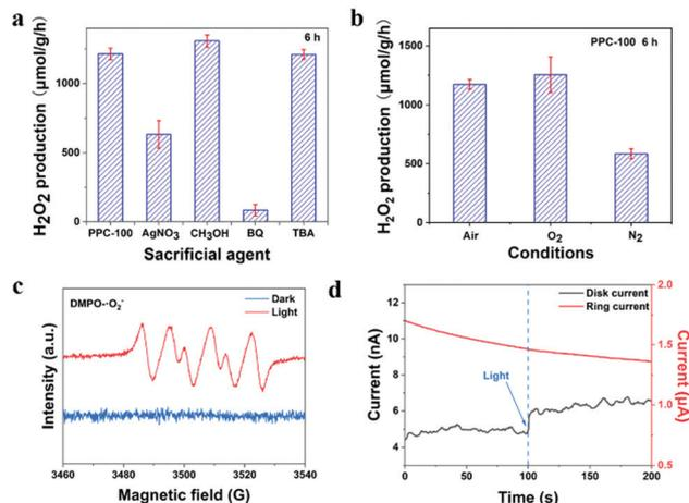
Fig. 8 (a)  $\text{H}_2\text{O}_2$  yield of catalyst PPC-100 which was added with different sacrificial agents. (b) The catalytic activity of catalysts under different atmospheres. (c) EPR spectra of catalyst PPC-100 to  $\cdot\text{O}_2^-$  under dark and light conditions. (d) The current–time curves of catalyst PPC-100.
