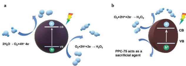
Fig. 9 (a) The mechanism diagram of photocatalytic  $\text{H}_2\text{O}_2$  production over the PPC-100 photocatalyst. (b) Possible mechanism diagram of photocatalytic  $\text{H}_2\text{O}_2$  production over the PPC-75 photocatalyst.
