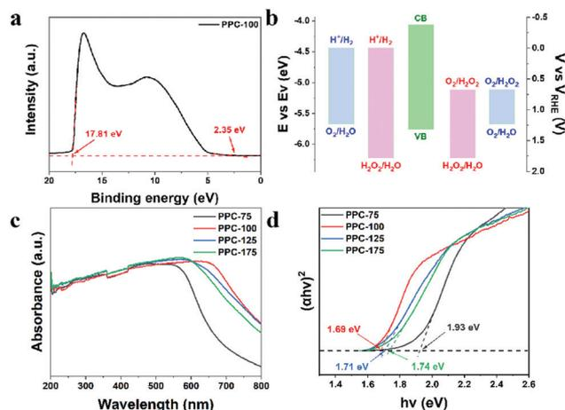
Fig. 3 (a) UPS spectrum of catalyst PPC-100. (b) Energy band structure of catalyst PPC-100 and the redox energy levels of water and  $\text{O}_2$ . (c) UV-Vis spectra and (d) the  $(\alpha h\nu)^2-h\nu$  curves of polymer catalysts PPC-X ( $X = 75, 100, 125, 175$ ).
