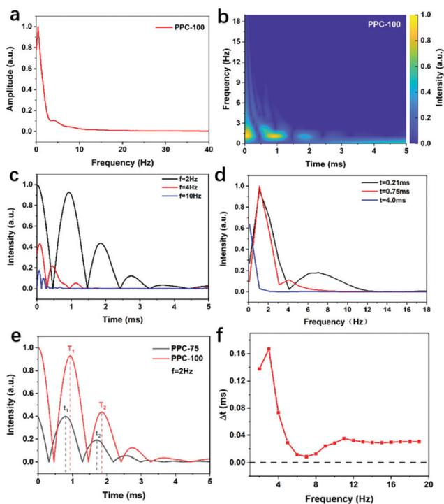
**Fig. 6** (a) FT spectrum, (b) 2D CWT spectrum, (c) Intensity–frequency curves ( $t = 0.21$ ,  $0.75$  and  $4.0$  ms) and (d) Intensity–time curves ( $f = 2$ ,  $4$ , and  $10$  Hz) of PPC-100, (e) Intensity–time curves of PPC-100, (f) Peak delay time ( $\Delta t$ ) at different frequencies ( $f = 2, 3, 4, 5, 6, 7, 8, 9, 10, 11, 12, 13, 14, 15, 16, 17$  and  $18$  Hz); here, the peak time of sample PPC-100 was used as the reference value.
