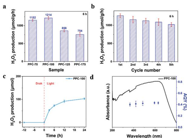
Fig. 7 (a)  $\text{H}_2\text{O}_2$  production rates of different PPC-X catalysts. (b) Cyclic stability of catalyst PPC-100. (c) Relation of  $\text{H}_2\text{O}_2$  yield of catalyst PPC-100 with time. (d) AQY of catalyst PPC-100 and its UV-Vis spectrum.
