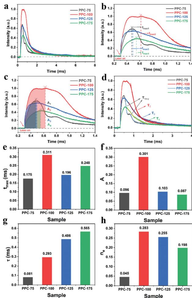
Fig. 5 (a) Comparison of the TPV with PPC-75, PPC-100, PPC-125 and PPC-175. (b) Maximum charge extraction time ( $t_{max}$ ) of PPC-75, PPC-100, PPC-125 and PPC-175. (c) Charge extraction of PPC-75, PPC-100, PPC-125 and PPC-175. (d) The charge recombination of PPC-75, PPC-100, PPC-125 and PPC-175. (e) Maximum charge extraction amount (A). (f) The maximum charge extraction (A). (g) Charge attenuation time ( $\tau$ ). (h) Surface effective charge ( $n_e$ ).
