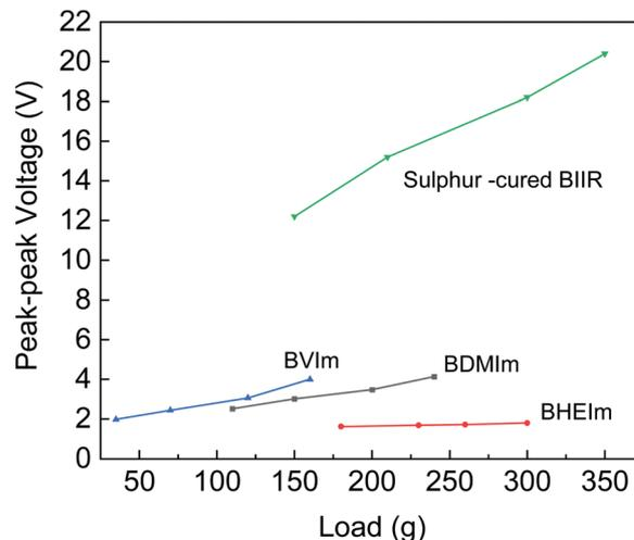
Fig. 9 The triboelectric performance of BIIR ionomers.
