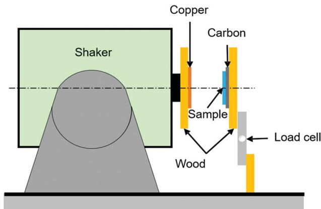
Fig. 1 Schematic of test setup to evaluate triboelectric properties.
