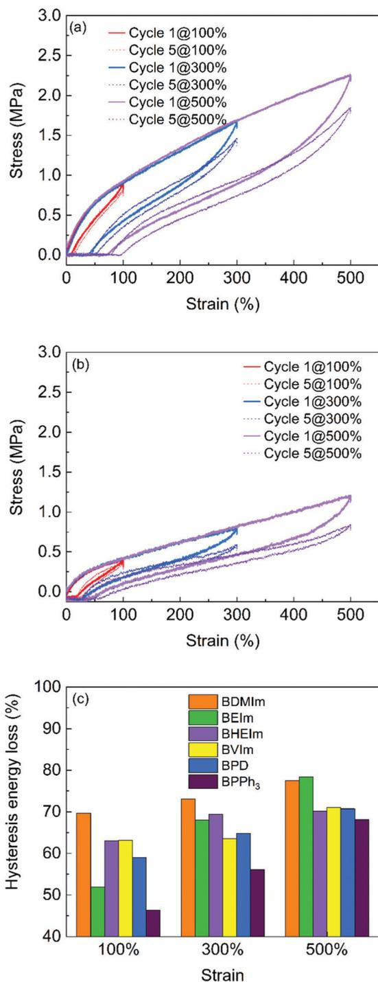
Fig. 8 Cyclic tensile testing of (a) BDMIm; (b) BPPH<sub>3</sub> with the maximum strain at 100%, 300% and 500% and (c) hysteresis energy loss of the BIIR ionomers after 5 cycles of extension.
