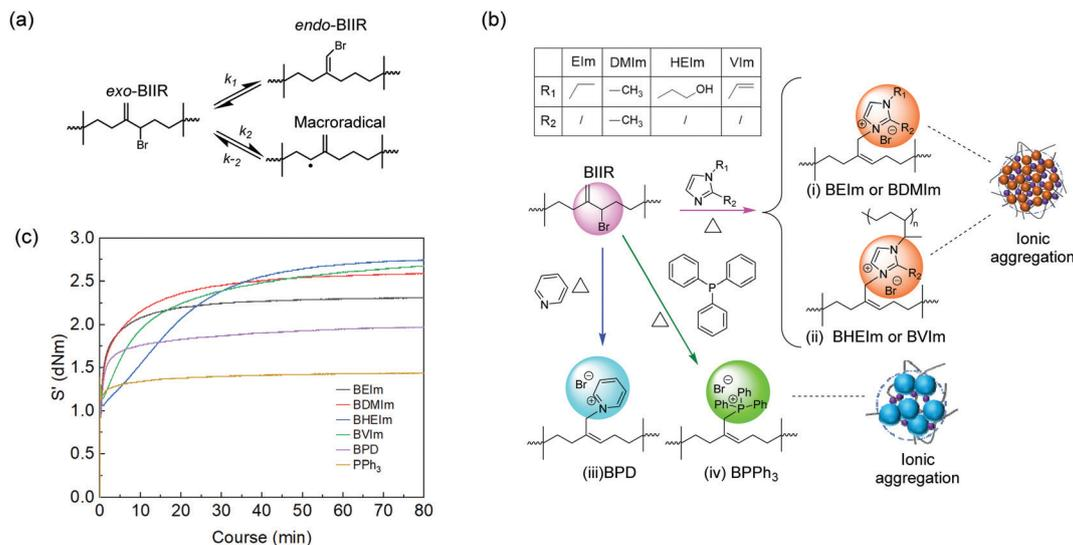
Fig. 3 (a) Schematic of main isomers and intermediates of BIIR rubber during heating; (b) schematic of synthesis of ionic modified BIIR using (i) alkyl imidazoles; (ii) 1-vinyl imidazole, structures shown in the inset table; (iii) pyridine; and (iv) triphenylphosphine; (c) monitoring the ionic clusters formation in different BIIR ionomers using a moving die rheometer.
