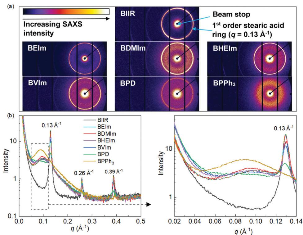
Fig. 5 (a) 2D SAXS data of all samples. The BIIR SAXS pattern shows labelling of the beam stop and the 1st order intense ring of the stearic acid at  $q = 0.13 \text{ \AA}^{-1}$ , and (b) 1D SAXS data of BIIR and ionomers and expanded area of the ionic aggregation peaks in ionomer samples (including the stearic acid 1st order peak at  $0.13 \text{ \AA}^{-1}$ ).
