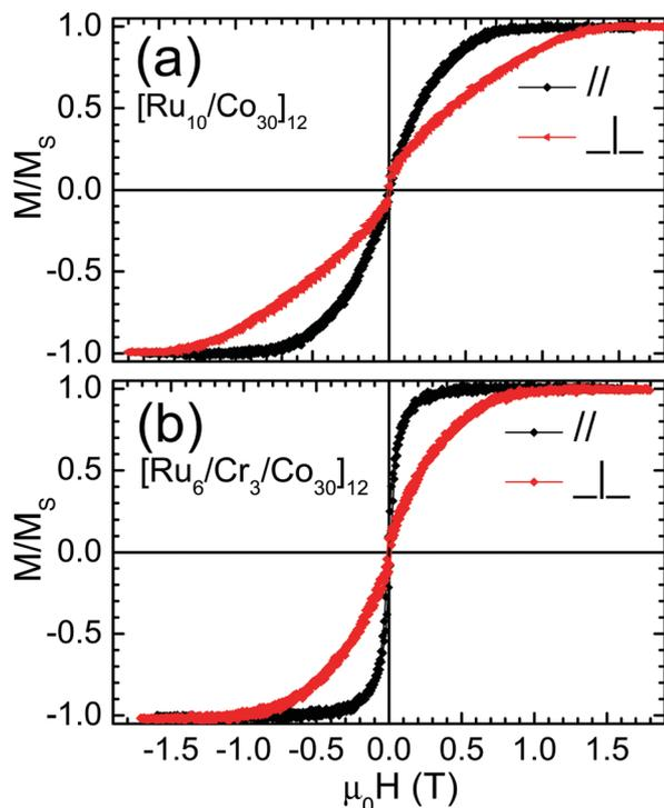
Fig. 1 Typical VSM magnetization curves for (a)  $[\text{Ru}_{10}/\text{Co}_{30}]_{12}$  and (b)  $[\text{Ru}_6/\text{Cr}_3/\text{Co}_{30}]_{12}$  samples. These curves are full loops from positive saturation to negative and back to positive. The paths of the two branches coincide.
