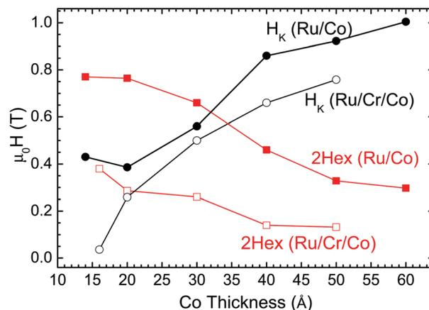
Fig. 2 Dependence of interlayer exchange field  $H_{\text{ex}}$  (squares) and anisotropy field  $H_{\text{K}}$  (circles) on Co layer thickness for  $[\text{Ru}_{10}/\text{Co}_{30}]_{12}$  (solid symbols) and (b)  $[\text{Ru}_6/\text{Cr}_3/\text{Co}_{30}]_{12}$  series (open symbols).
