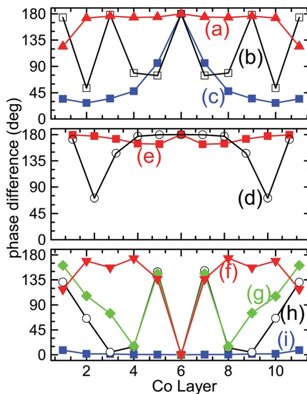
Fig. 6 Mode profiles: The phase difference of the precessional motion between consecutive cobalt layers for the points marked by the star symbols (a–i) in Fig. 5. The X-axis denotes the number  $n$  of the layer and the y axis the phase difference between the  $n$ -th and the  $(n + 1)$ -th layer. The profile (a) is closer to a pure optical mode whereas the profile (i) is closer to a pure acoustic mode. The rest of the profiles indicate a mixed character.
