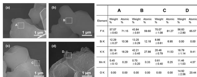
Fig. 7 SEM images and EDS results of the  $\text{H}_2\text{O}_2$ -treated water-resistant  $\text{K}_2\text{SiF}_6:\text{Mn}^{4+}$ : (a, A) before soaking in water and (b, B) after soaking in water for 6 h, and the SEM images and EDS results of the  $\text{K}_2\text{SiF}_6:\text{Mn}^{4+}$  prepared via the ionic exchange method: (c, C) before soaking in water and (d, D) after soaking in water for 6 h. Reprinted with permission from ref. 22 Copyright 2018 American Chemical Society.
