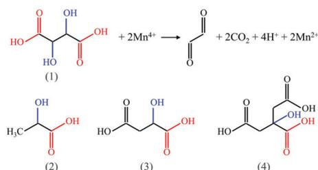
Fig. 9 Structural formulae of four  $\alpha$ -hydroxy acids: (1) tartaric acid, (2) lactic acid, (3) malic acid, and (4) citric acid, and the possible redox reaction between the tartaric acid and  $\text{Mn}^{4+}$  ion. Reprinted with permission from ref. 29 Copyright 2021 Elsevier.
