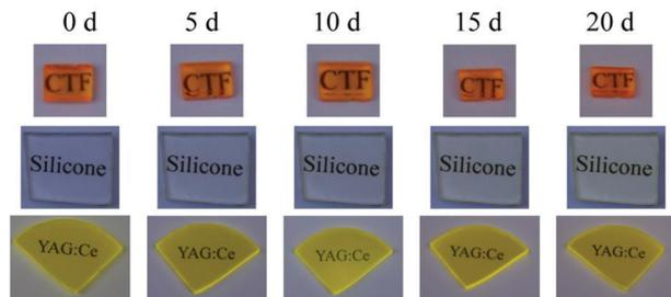
Fig. 14 Photographs of the  $\text{Cs}_2\text{TiF}_6\text{:Mn}^{4+}$  single crystal, silicone, and  $\text{Y}_3\text{Al}_5\text{O}_{12}\text{:Ce}^{3+}$  (YAG:Ce) crystal after heat treatment at  $150\text{ }^\circ\text{C}$  during different aging periods. Reprinted with permission from ref. 36 Copyright 2021 John Wiley and Sons.
