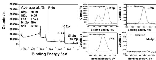
Fig. 8 X-ray photoelectron spectra (XPS) and high-resolution XPS of K 2p, Si 2p, F 1s, and Mn 2p of  $\text{H}_2\text{O}_2$ -treated water-resistant  $\text{K}_2\text{SiF}_6:\text{Mn}^{4+}$ . Reprinted with permission from ref. 22 Copyright 2018 American Chemical Society.
