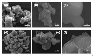
**Fig. 6** SEM images of the  $H_2O_2$ -treated water-resistant  $K_2SiF_6:Mn^{4+}$ : (a) before soaking in water and (b and c) after soaking in water for 6 h, and the SEM images of  $K_2SiF_6:Mn^{4+}$  prepared *via* the ionic exchange method: (d) before soaking in water and (e and f) after soaking in water for 6 h. Reprinted with permission from ref. 22 Copyright 2018 American Chemical Society.
