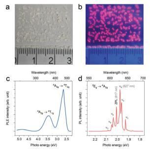
Fig. 11 Digital images of the  $Na_2SiF_6$  crystals doped with  $Mn^{4+}$ : (a) under daylight and (b) under 365 nm ultraviolent (UV) light. The photoluminescence excitation (monitoring for 627 nm emission) and emission (under 450 nm excitation) spectra were shown in (c) and (d), respectively. Reprinted with permission from ref. 34 Copyright 2021 John Wiley and
