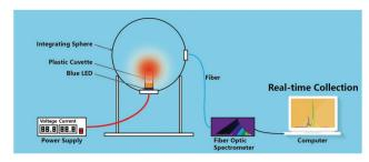
Fig. 13 Schematic of an apparatus including an integrating sphere and a fiber optic spectrometer which is recommended for use to record the photoluminescence intensity during the deterioration evaluation of Mn<sup>4+</sup>doped fluoride phosphors. Reprinted with permission from ref. 23 Copyright 2019 John Wiley and Sons.
