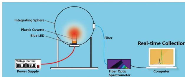
Fig. 13 Schematic of an apparatus including an integrating sphere and a fiber optic spectrometer which is recommended for use to record the photoluminescence intensity during the deterioration evaluation of  $\text{Mn}^{4+}$ -doped fluoride phosphors. Reprinted with permission from ref. 23 Copyright 2019 John Wiley and Sons.
