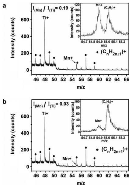
Fig. 3 Positive secondary ion mass spectra of the (a)  $\text{K}_2\text{TiF}_6:\text{Mn}^{4+}$  and (b)  $\text{K}_2\text{TiF}_6:\text{Mn}^{4+}@K_2\text{TiF}_6$  phosphors; insets show the enlarged peak of  $\text{Mn}^{4+}$ . Other peaks ( $\text{C}_n\text{H}_{2n\pm 1}^+$ , solid dots) originated from the conductive tape used for fixing phosphor powders. Reprinted with permission from ref. 20 Copyright 2019 John Wiley and Sons.
