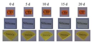
Fig. 14 Photographs of the  $Cs_2TiF_6$ : $Mn^{4+}$  single crystal, silicone, and  $Y_3Al_5O_{12}$ : $Ce^{3+}$  (YAG:Ce) crystal after heat treatment at 150 °C during different aging periods. Reprinted with permission from ref. 36 Copyright 2021 John Wiley and Sons.
