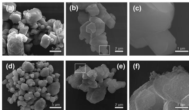
Fig. 6 SEM images of the  $\text{H}_2\text{O}_2$ -treated water-resistant  $\text{K}_2\text{SiF}_6:\text{Mn}^{4+}$ : (a) before soaking in water and (b and c) after soaking in water for 6 h, and the SEM images of  $\text{K}_2\text{SiF}_6:\text{Mn}^{4+}$  prepared via the ionic exchange method: (d) before soaking in water and (e and f) after soaking in water for 6 h. Reprinted with permission from ref. 22 Copyright 2018 American Chemical Society.
