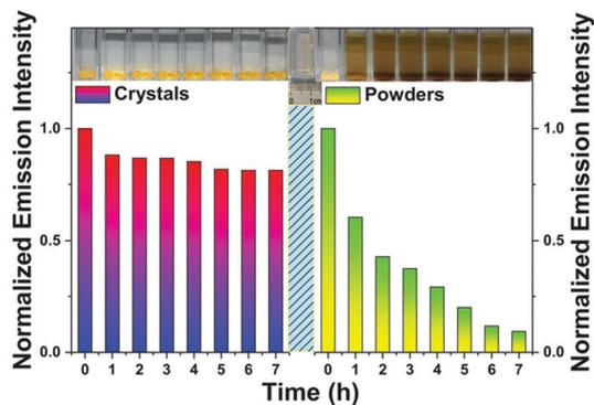
Fig. 10 Luminescence intensities of  $\text{Cs}_2\text{GeF}_6:\text{Mn}^{4+}$  crystals and powders measured after soaking in deionized water for different durations. Reprinted with permission from ref. 32 Copyright 2019 John Wiley and Sons.
