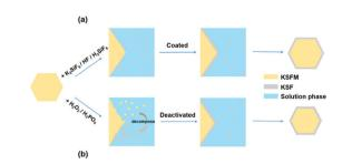
Fig. 5 Designing strategies for the K<sub>2</sub>SiF<sub>6</sub>:Mn<sup>4+</sup>@K<sub>2</sub>SiF<sub>6</sub> core-shell structure: (a) homogeneous coating and (b) surface deactivation. Reprinted with permission from ref. 22 Copyright 2018 American Chemical Society.
