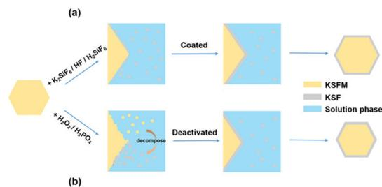
Fig. 5 Designing strategies for the  $\text{K}_2\text{SiF}_6:\text{Mn}^{4+}@K_2\text{SiF}_6$  core-shell structure: (a) homogeneous coating and (b) surface deactivation. Reprinted with permission from ref. 22 Copyright 2018 American Chemical Society.
