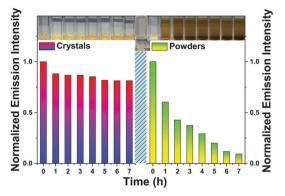
Fig. 10 Luminescence intensities of Cs<sub>2</sub>GeF<sub>6</sub>:Mn<sup>4+</sup> crystals and powders measured after soaking in deionized water for different durations. Reprinted with permission from ref. 32 Copyright 2019 John Wiley and Sons.
