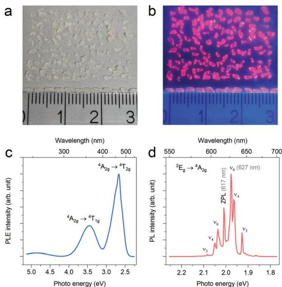
Fig. 11 Digital images of the  $\text{Na}_2\text{SiF}_6$  crystals doped with  $\text{Mn}^{4+}$ : (a) under daylight and (b) under 365 nm ultraviolet (UV) light. The photoluminescence excitation (monitoring for 627 nm emission) and emission (under 450 nm excitation) spectra were shown in (c) and (d), respectively. Reprinted with permission from ref. 34 Copyright 2021 John Wiley and Sons.
