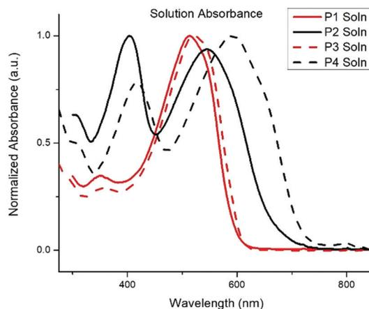
Fig. 1 Solution absorption profile of **P1–P4** with the concentration of  $10^{-5}$  M in chloroform.
