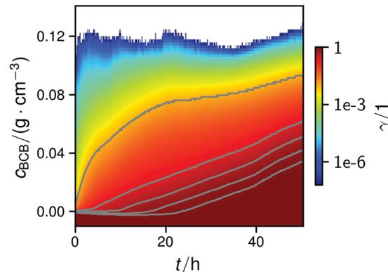
**Fig. 4** Map of the normalized cumulative histogram  $\gamma(C_{\text{BCB},b},t)$  at a flow rate of  $12.5 \text{ mm s}^{-1}$ . The gray plotted lines are isolines of  $\gamma = 0.01, 0.25, 0.50, 0.75,$  and  $0.9$ . They were fitted with a bi-logistic function  $C_{\text{BCB}}(\gamma,t)$ , eqn (4).
