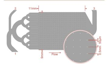
Fig. 2 Sketch of the microfluidic cell. The inoculum was injected into the larger inlet (1) from where it was evenly distributed into the inlet channels. This regularly allowed an even distribution of the fluid into the growth chamber, which was filled with evenly arranged obstacles with diameters of 50  $\mu m$  in 0.5 mm distance. After the growth, the smaller inlet (2) was used to add mineralisation medium. The inset shows a magnified section of the growth chamber.
