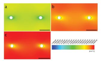
Fig. 10 Contour plots of the obstacles' surroundings at the flow rates 1.0 mm  $s^{-1}$  (a), 12.5 mm  $s^{-1}$  (b) and 25.0 mm  $s^{-1}$  (c) with flow from left to right.
