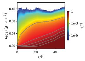
Fig. 4 Map of the normalized cumulative histogram  $\gamma(c_{BCB,b},t)$  at a flow rate of 12.5 mm s<sup>-1</sup>. The gray plotted lines are isolines of  $\gamma = 0.01$ , 0.25, 0.50, 0.75, and 0.9. They were fitted with a bi-logistic function  $c_{BCB}(\gamma,t)$ , eqn (4).
