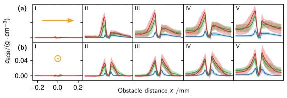
Fig. 8 Profile plots parallel (a) and perpendicular (b) to the flow in timesteps I-V of 7.5 h, where timestep I was 10 minutes after the start. The obstacle center is the x-axis center and fluid flow is indicated by the orange arrows. The blue line represents flow at 1.0 mm s<sup>-1</sup>, the green line at 12.5 mm s<sup>-1</sup> and the red line at 25.0 mm s<sup>-1</sup>.
