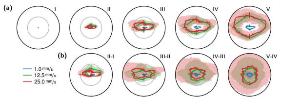
Fig. 7 Azimuthal plots of the obstacles' surroundings with the flow running from left to right in timesteps I-V of 7.5 h, whereby timestep I was 10 minutes after the start. Inner circles in row (a) represent a BCB concentration of 0.02 g cm<sup>-3</sup>, outer circles 0.04 g cm<sup>-3</sup>. Row (b) shows the differences between two timesteps from the upper row. Here, the inner circles represent 0.01 g cm<sup>-3</sup> and the outer circles 0.02 g cm<sup>-3</sup>.
