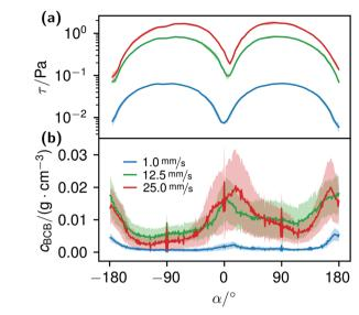
Fig. 11 Image (a) shows the calculated wall shear stress around nine parallel obstacles located in the middle of the microfluidic cell at different flow rates. In image (b) the azimuthal concentration  $c_{BCB}(\alpha)$  around the obstacles, 15 h after the start of the experiments, is pictured. The flow direction was from  $0^{\circ}$  to  $\pm 180^{\circ}$ .
