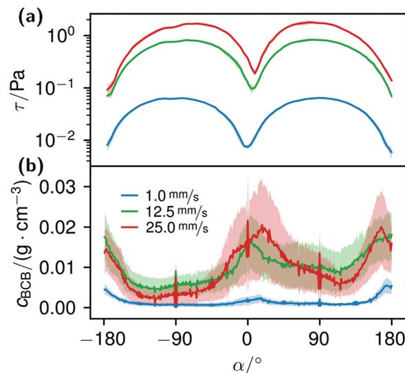
**Fig. 11** Image (a) shows the calculated wall shear stress around nine parallel obstacles located in the middle of the microfluidic cell at different flow rates. In image (b) the azimuthal concentration  $c_{\text{CCB}}(\alpha)$  around the obstacles, 15 h after the start of the experiments, is pictured. The flow direction was from  $0^\circ$  to  $\pm 180^\circ$ .
