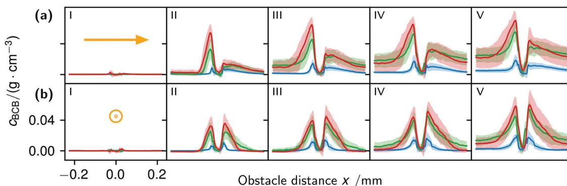
Fig. 8 Profile plots parallel (a) and perpendicular (b) to the flow in timesteps I–V of 7.5 h, where timestep I was 10 minutes after the start. The obstacle center is the  $x$ -axis center and fluid flow is indicated by the orange arrows. The blue line represents flow at  $1.0 \text{ mm s}^{-1}$ , the green line at  $12.5 \text{ mm s}^{-1}$  and the red line at  $25.0 \text{ mm s}^{-1}$ .
