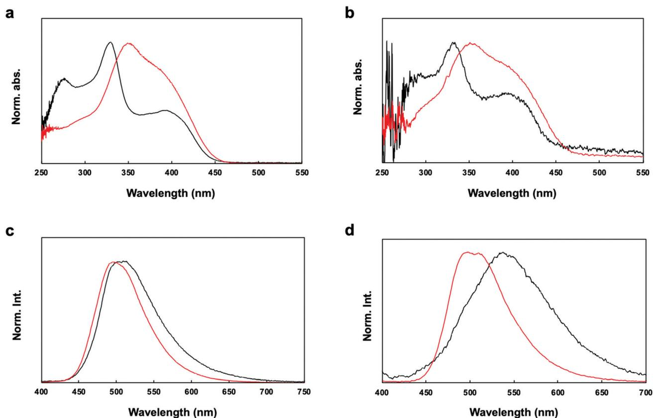
Fig. 4 Optical properties of the polymer. Black: **P1**. Red: **P2**. (a) UV-vis absorption spectra of the polymers in chloroform. (b) UV-vis absorption spectra of the polymers in film. (c) Fluorescence spectra of the polymers in chloroform. (d) Fluorescence spectra of the polymers in film.
