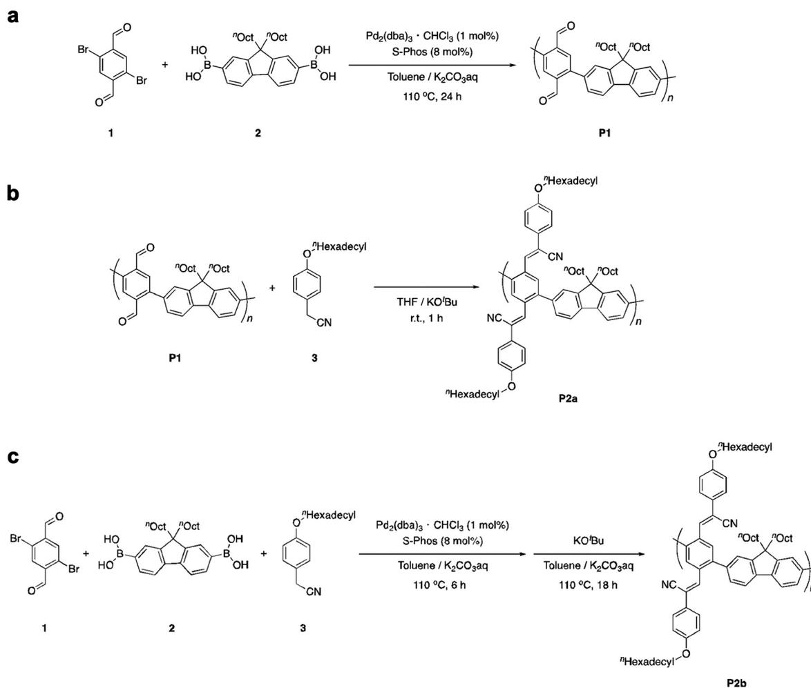
**Scheme 1** Synthetic strategy for  $\pi$ -conjugated polymers having an acrylonitrile side chain. (a and b) Post-polymerization process: synthesis of the polymers with an acrylonitrile unit in the side chain by Knoevenagel condensation on  $\pi$ -conjugated polymers with aldehyde. (c) One-pot process 2: synthesis of the polymer by step-wise Suzuki cross-coupling polycondensation and Knoevenagel condensation.
