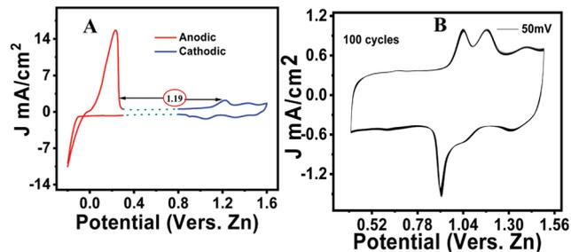
Fig. 3 (A) Voltammogram of zinc and pheno@cnt showing the cell voltage of 1.19 V. (B) Voltammogram showing the excellent stability of the electrode in 100 multiple sweep cycles at a 50 mV s<sup>-1</sup> scan rate.
