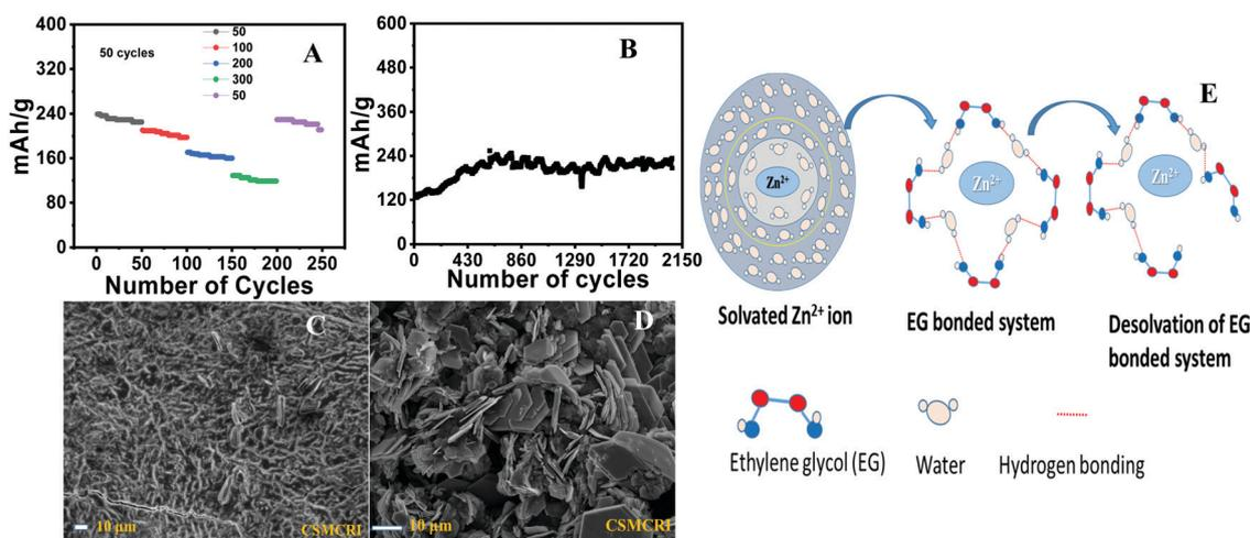
Fig. 8 (A) Rate stability test (fifty continuous cycles have been shown for each current density). (B) Prolonged cycling experiment for 2200 cycles at a current density of 300 mA g<sup>-1</sup>. Pheno@CNT in aqueous 2 M ZnSO<sub>4</sub>–ethylene glycol (1 : 1) electrolyte. (C and D) FESEM images of the anode and cathode surfaces after cycling. (E) Cartoon illustrating the solvated Zn<sup>2+</sup> ions as well as the ethylene glycol-associated solvation-desolvation mechanism.
