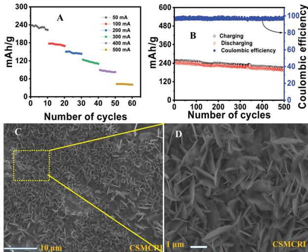
Fig. 7 (A) Rate stability test of the intercalated material at different currents (mA g<sup>-1</sup>). (B) Cycling stability test at 50 mA g<sup>-1</sup>. (C) FESEM images of the cathode. (D) The anode after the cycling experiment.
