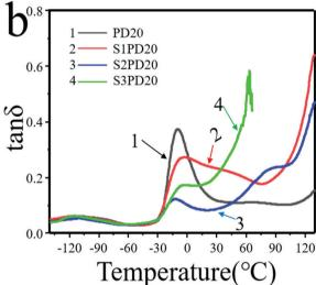
Fig. 5 Dynamic-mechanical spectra of the siloxane-based PCUs and their sulfobetaine modified ones. (a) E' and (b)  $\tan\delta$  vs. T.
