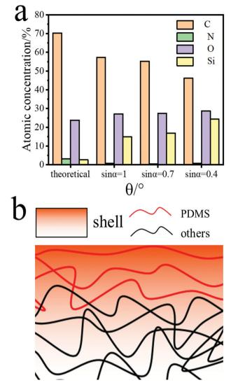
Fig. 6 XPS analysis of PD20 from different angles (a) and molecular model (b).
