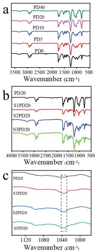
Fig. 2 FTIR spectra of the siloxane-based PCUs (a) and their sulfobetaine modified ones (b and c).
