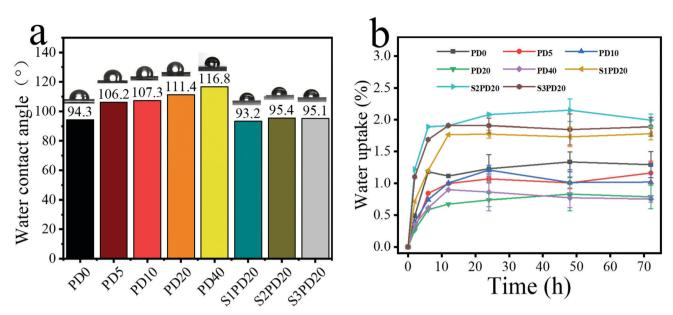
Fig. 7 Water contact angle of series polyurethane (a); water absorption curve of series polyurethane (b)
