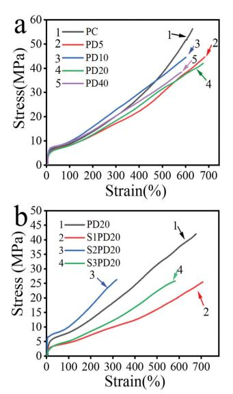
Fig. 4 Stress-strain curves of siloxane-based PC PUs (a) and their sulfobetaine modified ones (b).
