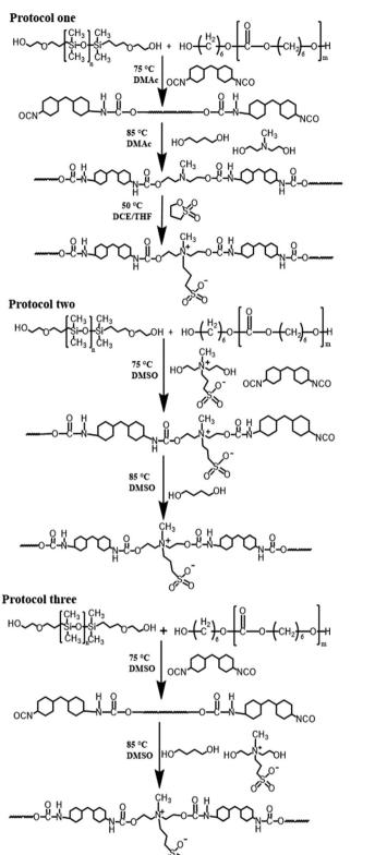
**Scheme 2** Synthetic pathways of sulfobetaine modified siloxane-based PCUs *via* three protocols.
