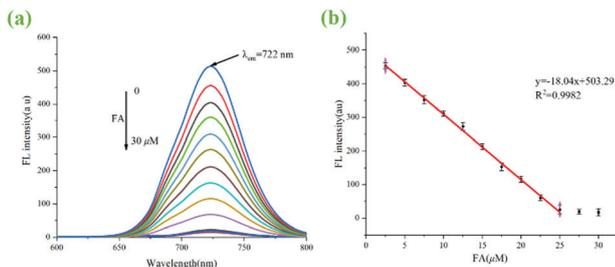
**Fig. 8** (a) The fluorescence spectra of **ZIF-90-Rhn@Ag<sup>+</sup>/Cy-N** in ethanol (100 μM/100 μM) with the addition of different concentrations of FA (0–30 μM). (b) The linear relationship between the fluorescence intensity and FA concentration.  $\lambda_{\text{ex}} = 678 \text{ nm}$ ,  $\lambda_{\text{em}} = 722 \text{ nm}$ .
