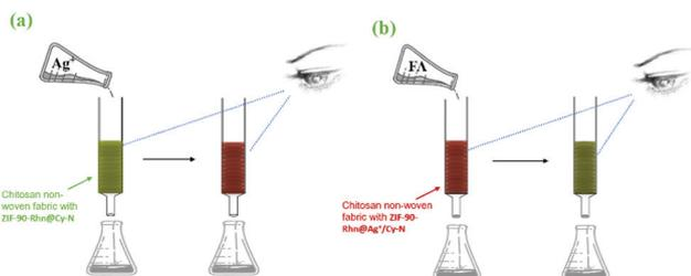
Fig. 16 (a) Schematic for the sensing and capturing of ZIF-90-Rhn@Cy-N toward Ag<sup>+</sup> in real samples. (b) The schematic for the sensing and capturing of ZIF-90-Rhn@Ag<sup>+</sup>/Cy-N toward FA in real samples.
