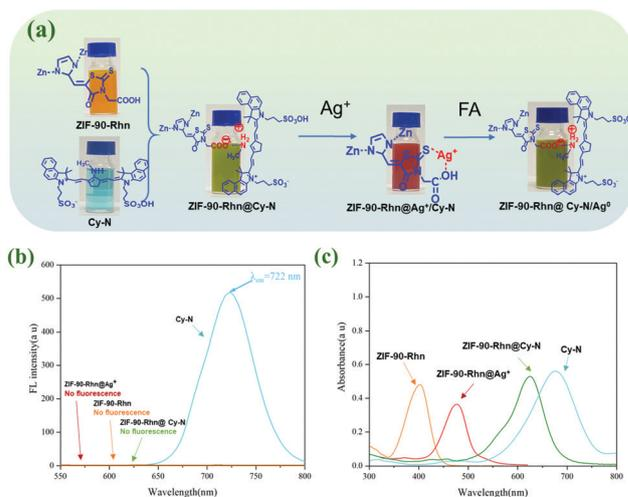
**Fig. 1** (a) Schematic representation of **ZIF-90-Rhn@Cy-N** for  $\text{Ag}^+$  and FA sensing. (The colors of all compounds were presented in ethanol solution.) (b) The fluorescence spectra of **ZIF-90-Rhn**, **ZIF-90-Rhn@Ag<sup>+</sup>**, **ZIF-90-Rhn@Cy-N** and **Cy-N** (100  $\mu\text{M}$  respectively),  $\lambda_{\text{ex}} = 678 \text{ nm}$ . (c) UV-vis spectra of **ZIF-90-Rhn**, **ZIF-90-Rhn@Ag<sup>+</sup>**, **ZIF-90-Rhn@Cy-N** and **Cy-N**.
