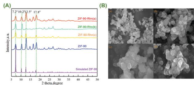
**Fig. 3** (A) PXRD data of **ZIF-90-Rhn** (a–c), **ZIF-90** and the simulated pattern of **ZIF-90**. (B) (a) SEM images of **ZIF-90**; (b) SEM images of **ZIF-90-Rhn** (a); (c) SEM images of **ZIF-90-Rhn** (b); (d) SEM images of **ZIF-90-Rhn** (c).
