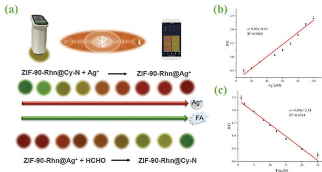
**Fig. 10** (a) The RGB analysis for the color changes of **ZIF-90-Rhn@Cy-N** in ethanol (100 μM) corresponding to Ag<sup>+</sup> (10–100 μM) and **ZIF-90-Rhn@Ag<sup>+</sup>/Cy-N** in ethanol (100 μM/100 μM) to FA (1–25 μM) using the smartphone and spectrophotometer portable detection platform. (b) The linear relationship between the R/G values and the Ag<sup>+</sup> concentrations in RGB analysis. (c) The linear relationship between the R/G values and the FA concentrations in RGB analysis.
