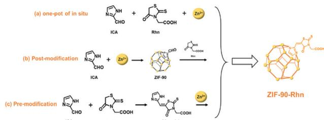
**Scheme 1** The synthetic route of **ZIF-90-Rhn**. (The end product through *in situ* synthesis was named **ZIF-90-Rhn** (a), the end product through post-modification was named **ZIF-90-Rhn** (b), the end product through pre-modification was named **ZIF-90-Rhn** (c).)
