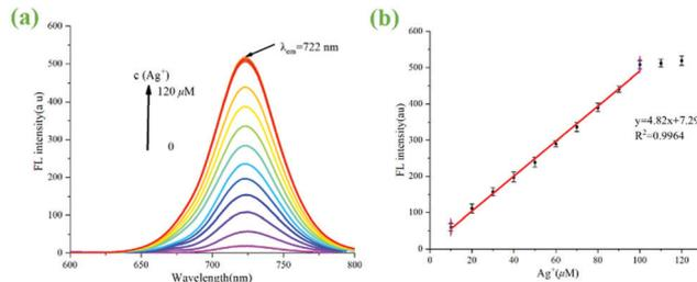
Fig. 6 (a) The fluorescence spectra of ZIF-90-Rhn@Cy-N in ethanol (100 μM) with the addition of different concentrations of Ag<sup>+</sup> (0–120 μM). (b) The linear relationship between the fluorescence intensity and Ag<sup>+</sup>.  $\lambda_{\text{ex}} = 678 \text{ nm}$ ,  $\lambda_{\text{em}} = 722 \text{ nm}$ .
