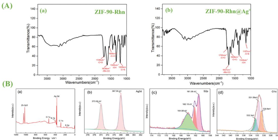
Fig. 15 (A-a) FT-IR spectra of ZIF-90-Rhn; (A-b) FT-IR spectra of ZIF-90-Rhn@Ag<sup>+</sup>; (B) XPS spectra of ZIF-90-Rhn@Ag<sup>+</sup> sample: (a) the survey scan; (b) Ag 3d; (c) S 2p; (d) O 1s.
