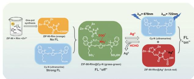
Fig. 13 Schematic illustration of **ZIF-90-Rhn@Cy-N** structure and visual detection principle for **Ag<sup>+</sup>** and FA.
