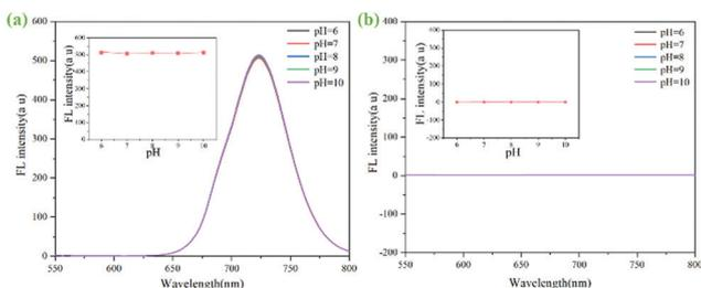
Fig. 5 (a) Fluorescence spectra changes of ZIF-90-Rhn@Cy-N (100 μM) response to Ag<sup>+</sup> (100 μM) in different pH. (b) Fluorescence spectra changes of ZIF-90-Rhn@Ag<sup>+</sup>/Cy-N (100 μM) response to FA (25 μM) in different pH.  $\lambda_{\text{ex}} = 678 \text{ nm}$ ,  $\lambda_{\text{em}} = 722 \text{ nm}$ .
