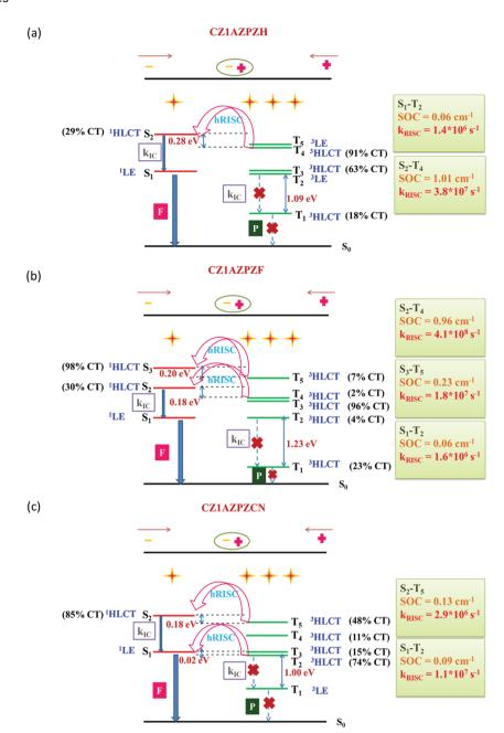
Fig. 5 Schematic depiction of a favourable hRISC process in (a) CZ1AZPZH, (b) CZ1AZPZF and (c) CZ1AZPZCN with the calculated energy levels, accompanying SOCs, and associated  $k_{RISC}$ .
