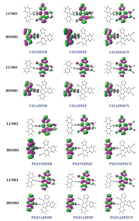
Fig. 3 The HOMO-LUMO wavefunctions of the studied molecules at ωB97X/6-31G(d,p) level of theory.
