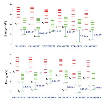
Fig. 4 Excited state energy diagrams of molecules, including the lowest ten singlet and ten triplet excited states at TDA/ωB97X/6-31G(d,p) level of theory
