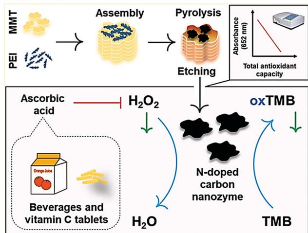
Fig. 10 N-Doped carbon as a peroxidase-like catalyst for the detection of  $\text{H}_2\text{O}_2$ , glucose, and ascorbic acid.<sup>163</sup> Copyright American Chemical Society 2019.
