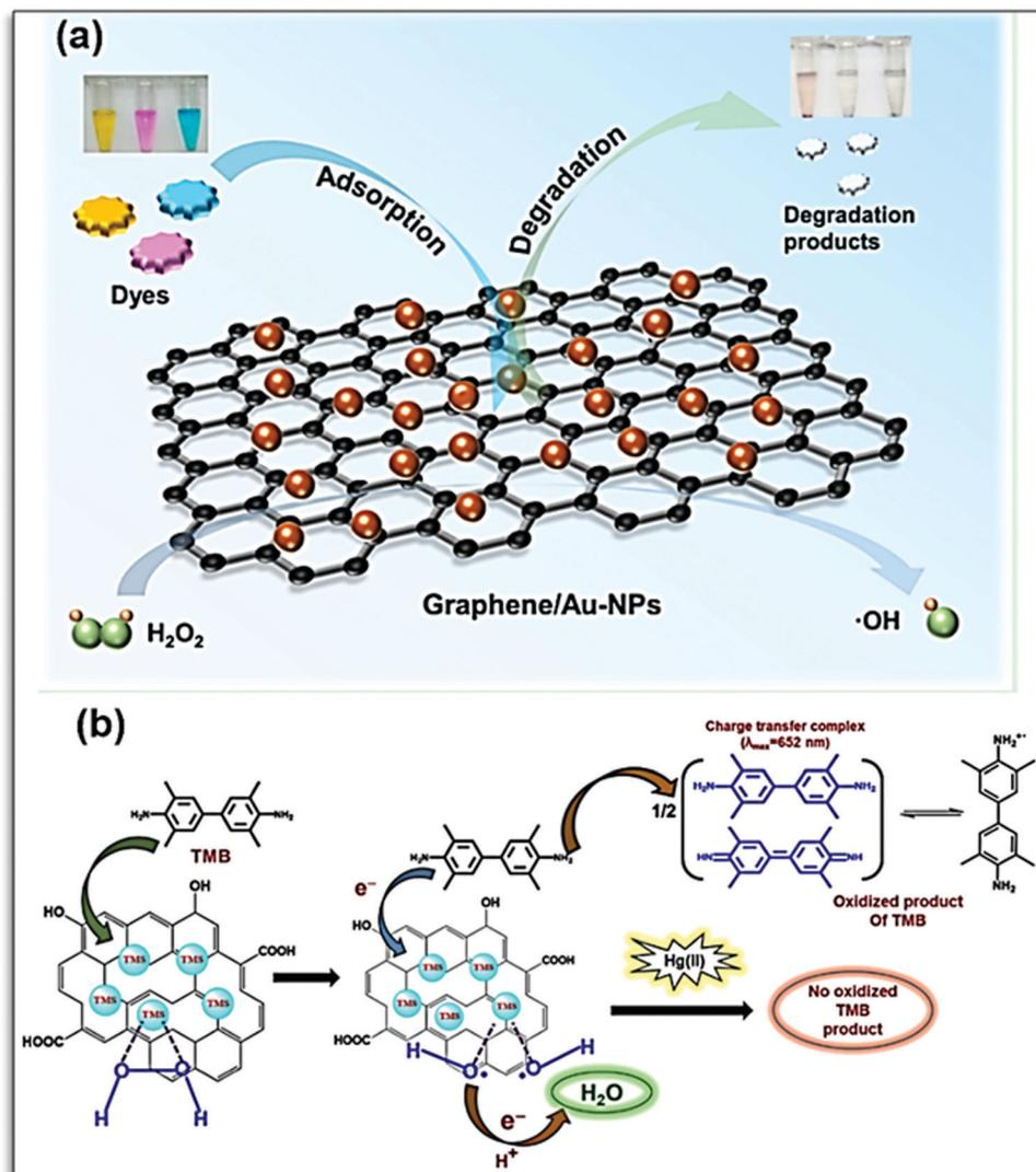
Fig. 13 (a) Schematic representation of the peroxidase-mimicking activity of graphene/Au-NPs for the adsorption and degradation of dyes.<sup>182</sup> (b) Mechanism of peroxidase-mimicking activity of transition metal sulfide (TMS)/p-rGO nanocomposites in the presence and absence of  $Hg(II)$  ions.<sup>183</sup> Copyright American Chemical Society 2021.
