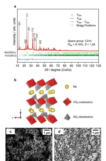
Fig. 2 (a) XRD pattern and the results of the Rietveld refinement of the as-prepared NaV( $SO_4$ )<sub>2</sub>. (b) The crystal structure obtained from the Rietveld-refined NaV( $SO_4$ )<sub>2</sub>. The structure was visualized using VESTA. SEM images of the (c) as-prepared NaV( $SO_4$ )<sub>2</sub> and (d) carbon-coated NaV( $SO_4$ )<sub>2</sub> prepared by ball milling.
