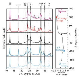
Fig. 4  $Ex\ situ\ XRD\$ patterns during galvanostatic measurements using 1 M NaClO $_4$  in EC:DMC (1:1 by volume) as the electrolyte for the initial state (black line), the desodiation/sodiation process (red and pink lines), and the sodiation/desodiation process (blue and light-blue lines). Black and white star icons show the new diffraction peaks on the discharging and charging process, respectively.
