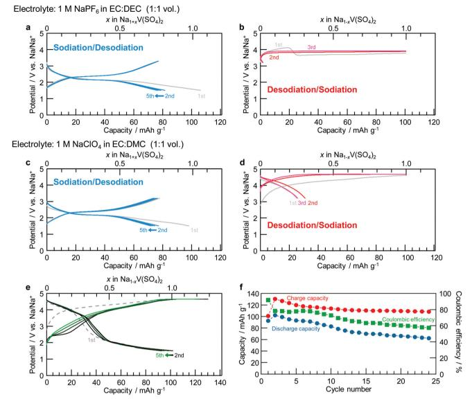
Fig. 3 Charge-discharge profiles of NaV(SO<sub>4</sub>)<sub>2</sub> showing sodiation and desodiation in cells prepared with two different electrolytes: (a) and (b) 1 M NaPF<sub>6</sub> in EC: DEC (1:1 by volume) and (c) and (d) 1 M NaClO<sub>4</sub> in EC: DMC (1:1 by volume). (e) Charge-discharge profiles and (f) cycle performance of NaV(SO<sub>4</sub>)<sub>2</sub> in the voltage region of 1.5-4.8 V; the electrolyte was 1 M NaClO<sub>4</sub> in EC: DMC (1:1 by volume).
