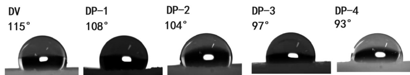
Fig. 4 Water contact angle of DV and the DP adsorbent.
