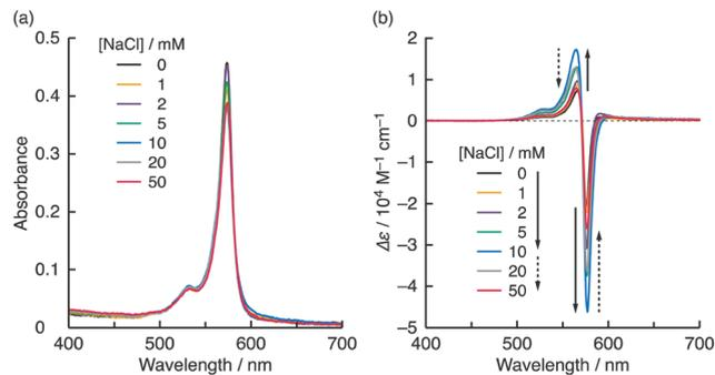
**Fig. 3** (a) Visible absorption and (b) CD spectra of NK-77 (0.01 mM) in the presence of L-1 (0.2 mM) in water at pH 10 containing various NaCl concentrations at 20 °C; path length: 0.1 cm. Variations in absorbance and  $\Delta\epsilon$  as functions of NaCl concentration are shown in Fig. S7 (ESI<sup>†</sup>).
