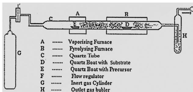
Fig. 1 Schematic diagram of CVD set up.
