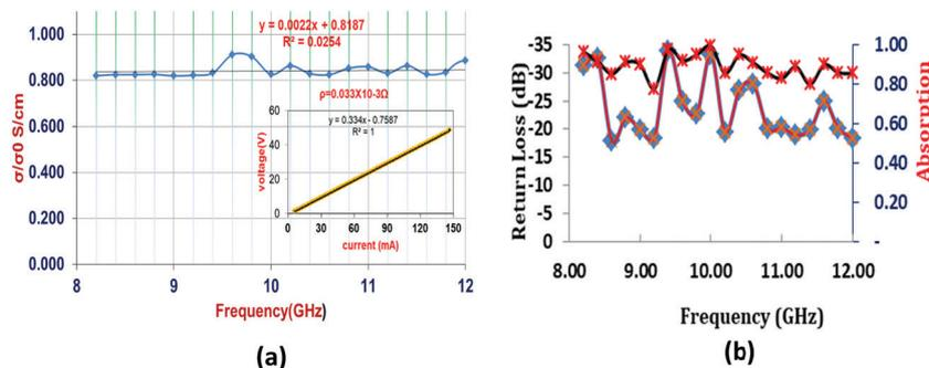
Fig. 3 (a) Microwave conductivity against frequency along with electrical resistance plot for CNFs film (b) Microwave absorption and return loss vs. frequency curve for CNFs film.
