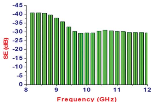
Fig. 4 Shielding effectiveness vs. frequency plot for CNFs.
