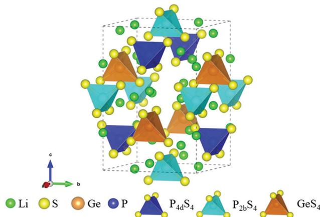
Fig. 1 Crystal structure of  $\text{Li}_{10}\text{GeP}_2\text{S}_{12}$ .
