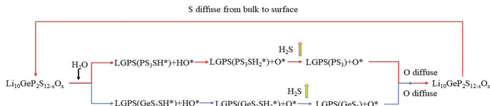
Fig. 3 Reaction paths of  $\text{Li}_{10}\text{GeP}_2\text{S}_{12}$  surfaces and  $\text{H}_2\text{O}$ , where the red path represents  $\text{H}_2\text{O}$  reacting with S in the  $\text{PS}_4$  tetrahedra, and the blue one represents  $\text{H}_2\text{O}$  reacting with S in the  $\text{GeS}_4$  tetrahedra.
