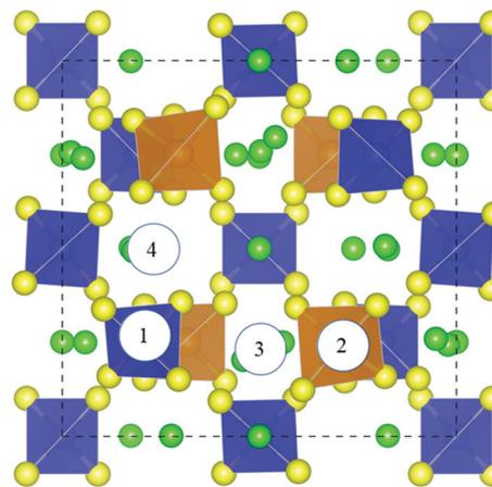
Fig. 2  $\text{H}_2\text{O}$  adsorption site on the  $\text{Li}_{10}\text{GeP}_2\text{S}_{12}$ (110) surface. Site ① is the adsorption site on the  $\text{PS}_4$  tetrahedron, site ② is the adsorption site on the  $\text{GeS}_4$  tetrahedron, and sites ③ and ④ are the adsorption sites on  $\text{Li}^+$ .
