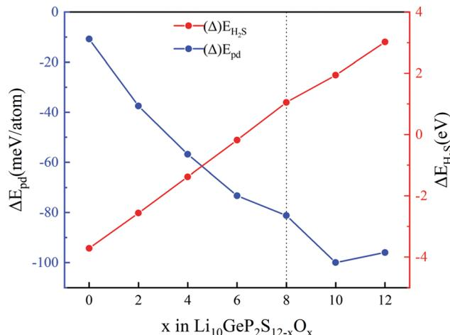
**Fig. 7** Phase decomposition (pd) stability ( $\Delta E_{\text{pd}}$ , reaction equilibrium in eqn (5)–(8) and moisture stability with  $x$  in the  $\text{Li}_{10}\text{GeP}_2\text{S}_{12-x}\text{O}_x$ .
