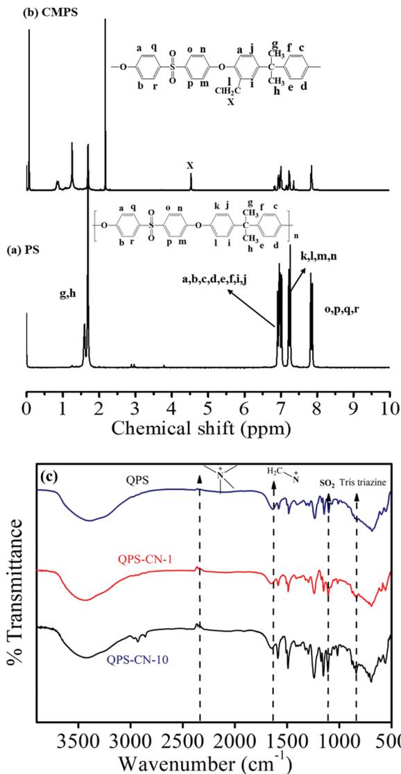
Fig. 3 (a, b) <sup>1</sup>H NMR of PS (polysulfone) and CMPS (chloromethylated polysulfone). (c) FT-IR spectra of QPS, QPS-CN-1 and QPS-CN-10.
