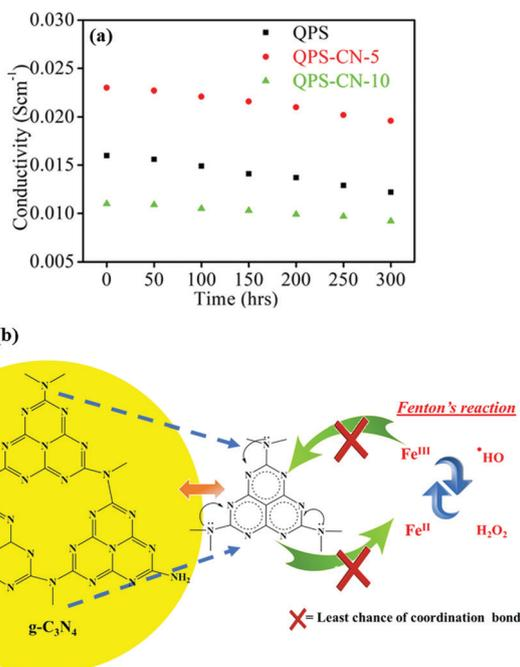
Fig. 8 (a) Alkaline stability of the QPS and QPS-CN<sub>x</sub> composite membranes in 3 M NaOH for 300 h and (b) the related mechanism showing the stability against Fenton's reagent.
