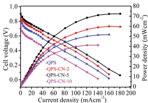
**Fig. 9** Cell performance of the QPS and QPS-CN<sub>x</sub> composite membranes at a 300 cm<sup>3</sup> min<sup>-1</sup> H<sub>2</sub>/O<sub>2</sub> flow rate under 100% RH.
