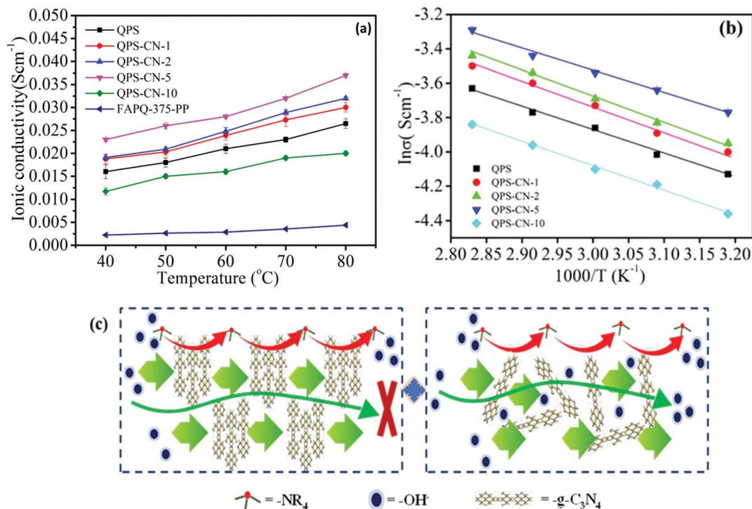
Fig. 6 (a) Temperature dependence of ionic conductivity and (b) its Arrhenius behavior for the QPS and QPS-CN<sub>x</sub> composite membranes. (c) The proposed mechanism for improved ionic conductivity.
