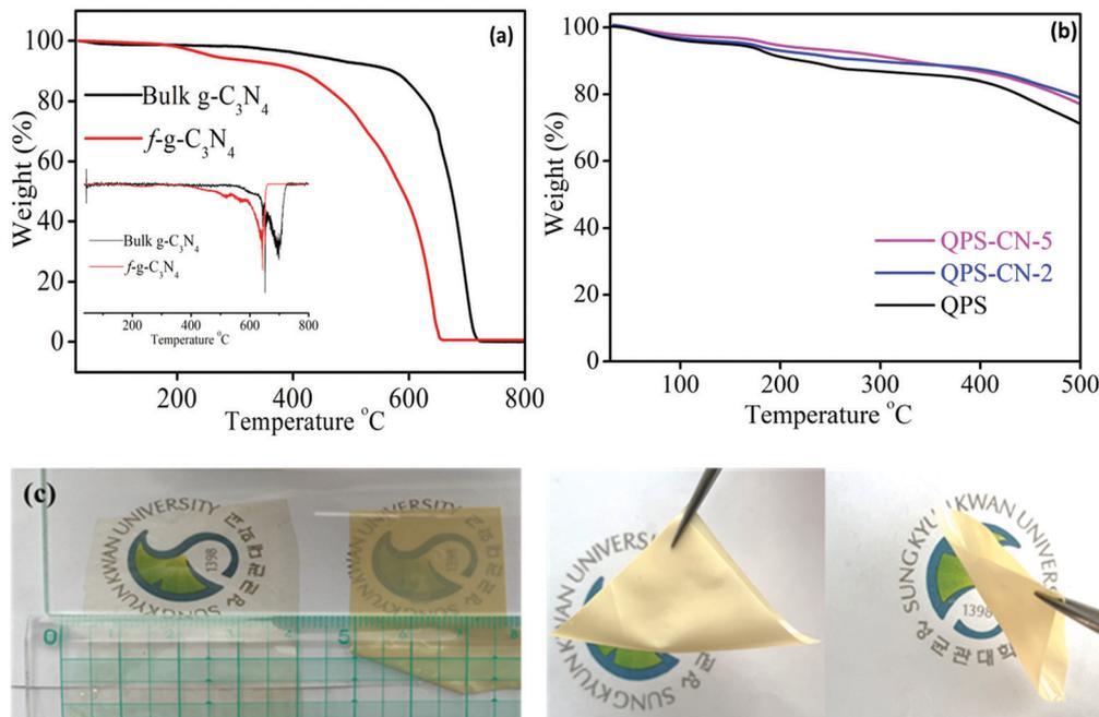
Fig. 5 TGA behavior of the (a) bulk and functionalized  $g\text{-C}_3\text{N}_4$  (dTg spectra inserted) and (b) QPS and QPS-CN $_x$  membranes. (c) Optical images of the QPS and QPS-CN-5 membranes.
