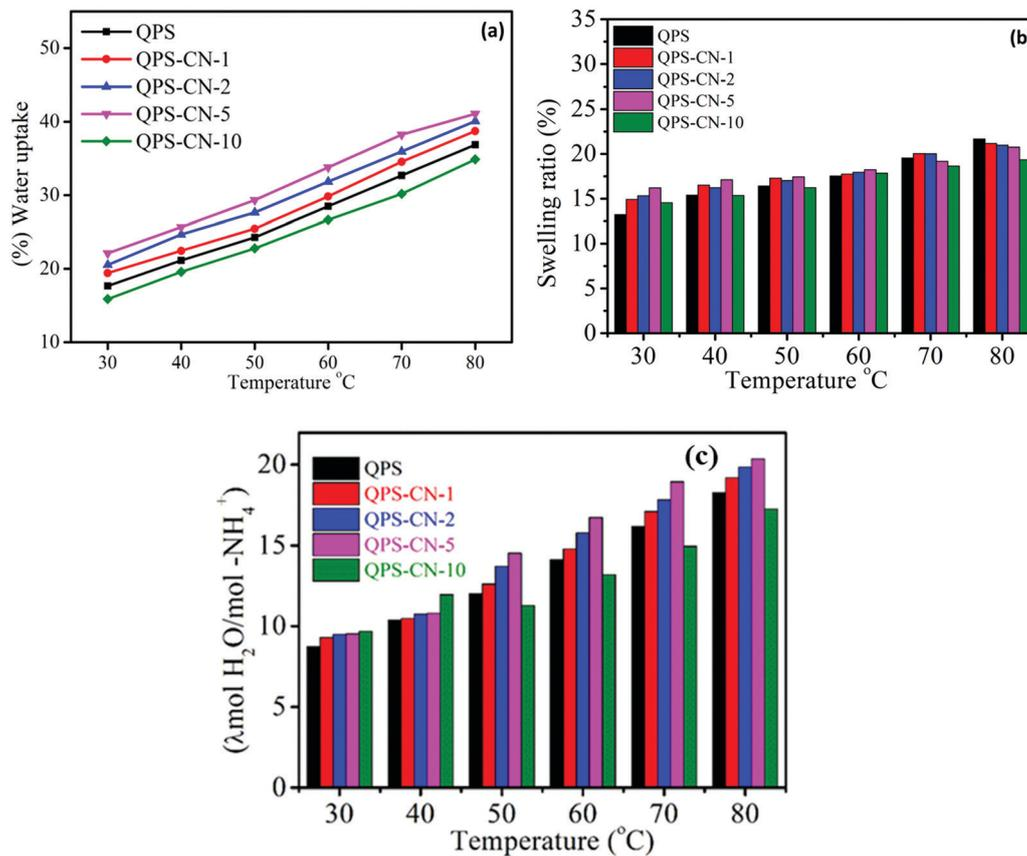
Fig. 7 (a) Water uptake, (b) swelling ratio, and (c) hydration number of the QPS and QPS-CN<sub>x</sub> composite membranes at different temperatures.
