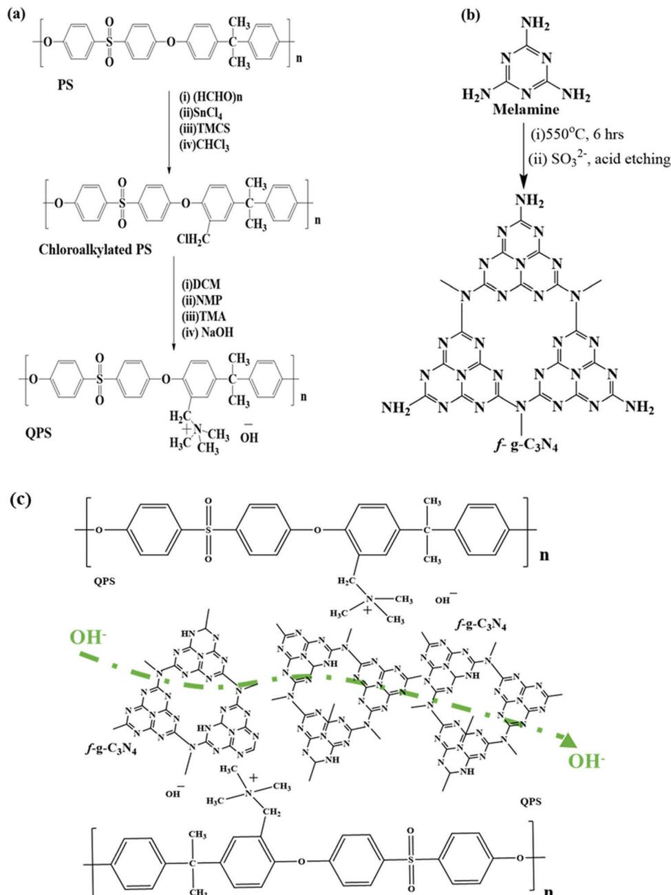
Scheme 1 Synthetic schemes of (a) QPS, (b)  $f\text{-}g\text{-C}_3\text{N}_4$ , and (c) QPS-CN<sub>x</sub>.
