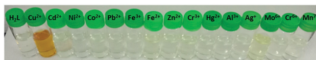
Fig. 3 Colour change in visible light of probe H 2 L on addition of different metal ions.
