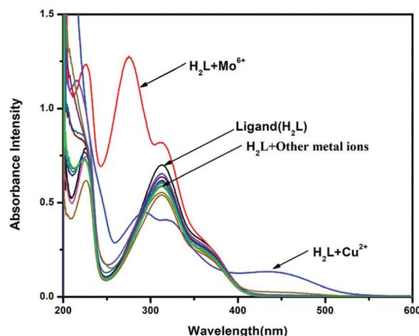
Fig. 4 Absorption spectra of **H<sub>2</sub>L** (10 μM) changes in the presence of 5 equiv. of different metal ions.
