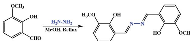
Scheme 1 Synthesis of the probe H<sub>2</sub>L.
