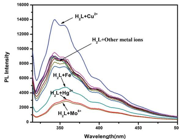
Fig. 9 Fluorescence spectra of  $\text{H}_2\text{L}$  with different cations.
