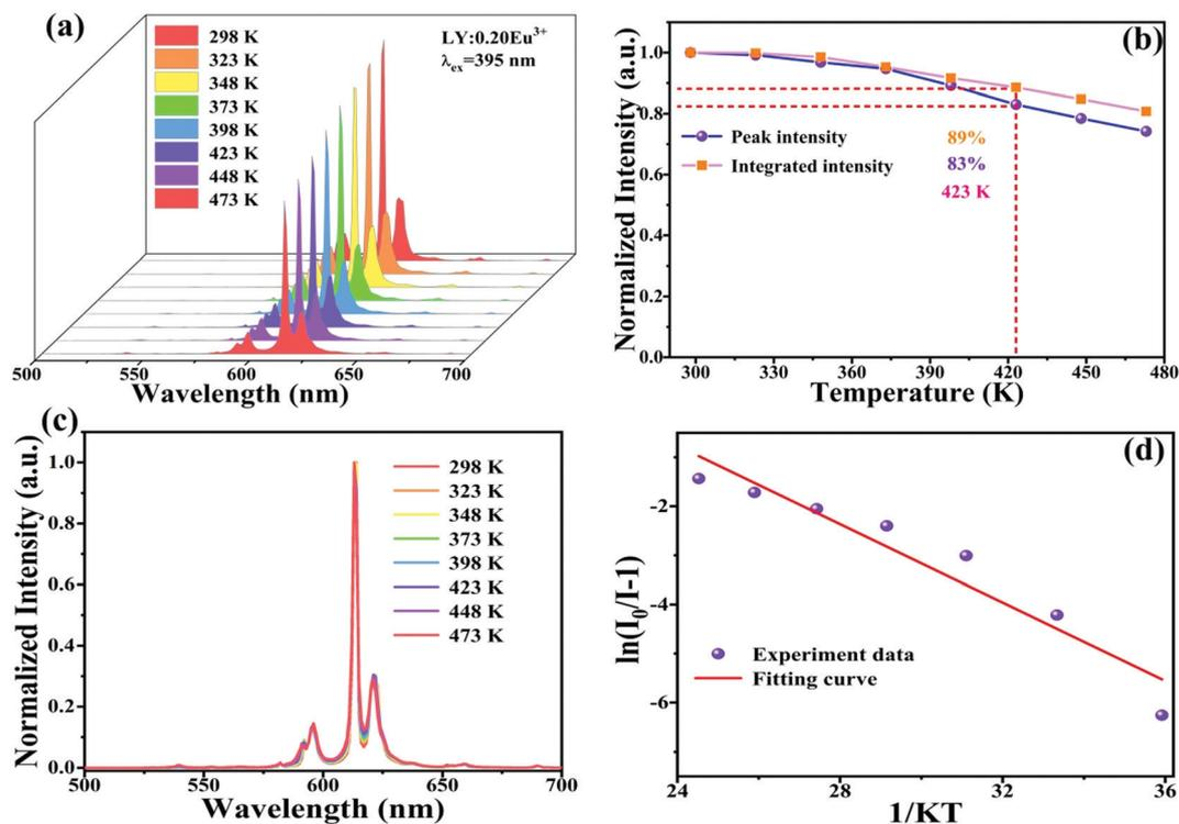
Fig. 6 (a)–(c) PL spectra, the relative peak and integrated intensity, and normalized PL spectra at different temperatures (298–473 K) of the  $\text{LiYO}_2:0.20\text{Eu}^{3+}$  sample. (d) The linear relationship of  $\ln(I_0/I-1)$  with  $1/KT$ .
