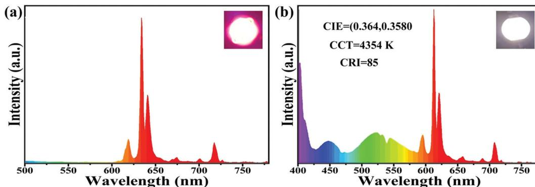
Fig. 7 Electroluminescence spectra and photographs of (a) n-UV LED chip +  $\text{LiYO}_2:0.20\text{Eu}^{3+}$  phosphor and (b) n-UV LED chip +  $\text{BaMgAl}_{10}\text{O}_{17}:\text{Eu}^{2+}$  +  $(\text{Sr}, \text{Ba})_2\text{SiO}_4:\text{Eu}^{2+}$  +  $\text{LiYO}_2:0.20\text{Eu}^{3+}$ .
