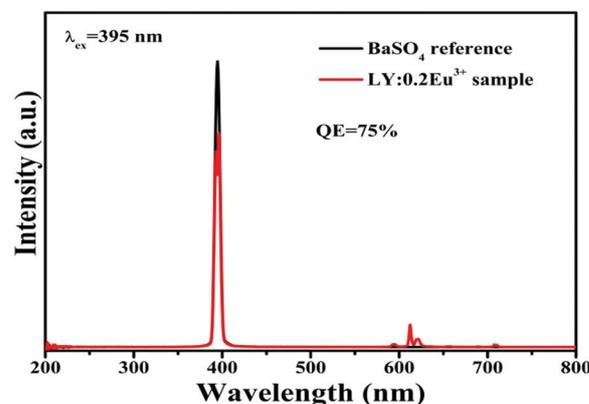
Fig. 5 Quantum efficiency of the  $\text{LY}:0.20\text{Eu}^{3+}$  phosphor.
