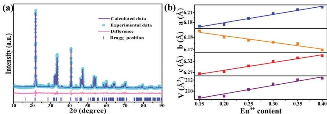
Fig. 2 (a) The Rietveld refinements of  $\text{LiYO}_2:0.20\text{Eu}^{3+}$  and (b) the relationship between lattice parameters and the differing amounts of  $\text{Eu}^{3+}$  in the  $\text{LiYO}_2$  host.
