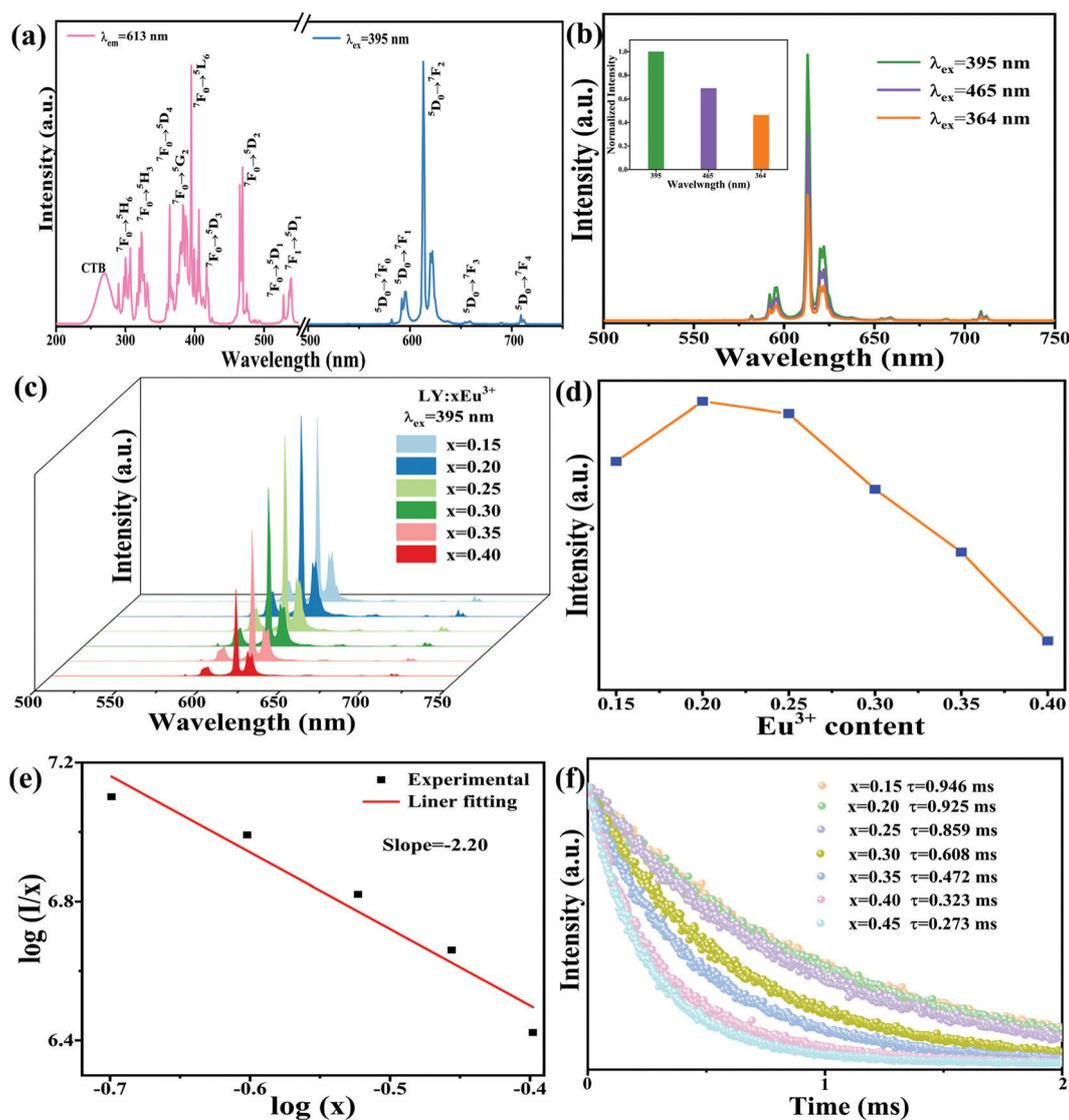
Fig. 3 (a) and (b) Excitation and emission spectra with different excitation wavelengths of  $\text{LiYO}_2:xEu^{3+}$ . (c) Emission spectra for different concentrations of  $\text{Eu}^{3+}$  and (d) relative intensity of the  $\text{LiYO}_2:xEu^{3+}$  samples. (e) Dependence of  $\log(I/x)$  with  $\log(x)$ . (f) The PL decay curves of  $\text{LiYO}_2:xEu^{3+}$ .
