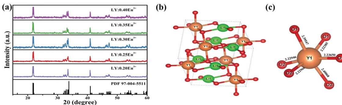
Fig. 1 (a) XRD patterns of  $\text{LiYO}_2:x\text{Eu}^{3+}$  ( $x = 0.20$ – $0.40$ ) and the standard XRD card (PDF No. 97-004-5511). (b) The unit cell structure of  $\text{LiYO}_2$  and (c) the bond lengths of the  $\text{YO}_6$  octahedra.
