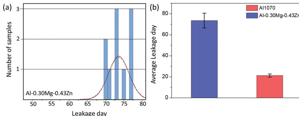
Fig. 10 (a) The leakage day data of the Al-0.30Mg-0.43Zn alloy. (b) The histogram of the leakage day data of Al1070 and alloy Al-0.30Mg-0.43Zn.
