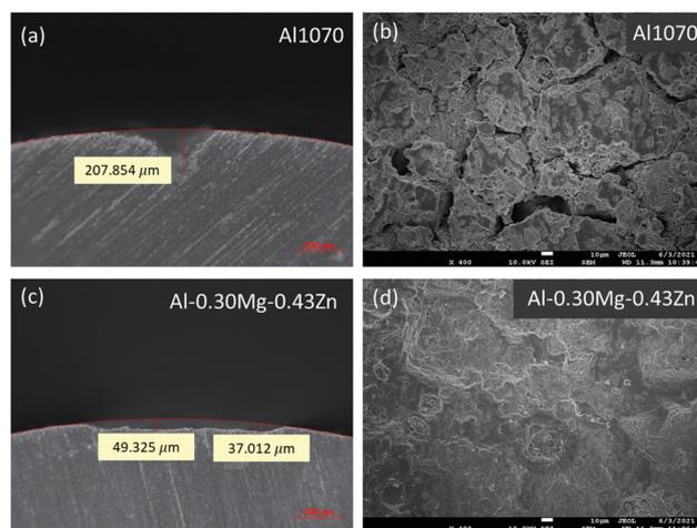
Fig. 8 Optical microscope image showing the pitting depth of each sample after the 15 days SWAAT experiment: (a) Al 1070 and (c) Al–0.30Mg–0.43Zn. SEM image showing the surface of (b) Al 1070 and (d) Al–0.30Mg–0.43Zn.
