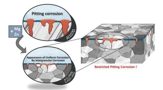
Scheme 1 The addition of Mg and Zn to Al1070 changed the pitting form of corrosion to the appearance of uniform corrosion by intergranular corrosion and increased corrosion resistance
