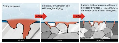
Scheme 2 The schematic representation of the change in corrosion from pitting to intergranular corrosion on adding Mg and Zn with the Al1070 alloy.
