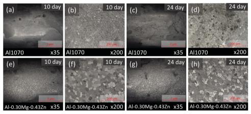
Fig. 4 Surface view observation of the corroded specimens after the SWAAT; (a and b) Al 1070 on the 10th day of the SWAAT experiment. (c and d) Al 1070 on the 24th day of the SWAAT experiment. (e and f) Al-0.30Mg-0.43Zn on the 10th day of the SWAAT experiment. (g and h) Al-0.30Mg-0.43Zn on the 24th day of the SWAAT experiment.
