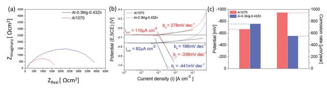
Fig. 9 (a) Nyquist impedance plot of electrochemical impedance spectroscopy (EIS), (b) potentiodynamic polarization curves, and (c) the potential and corrosion rate graph.
