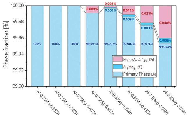
Fig. 2 Phase fraction calculation data of Al-xMg-yZn (0.10 < wt% of x < 1.00, 0.10 < wt% of y < 0.55) samples.
