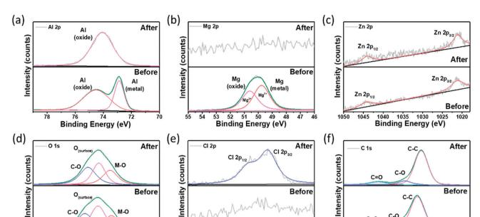
Fig. 7 X-Ray photoelectron spectroscopy scans of the Al-Mq-Zn alloy: (a) Al 2p, (b) Mq 2p, (c) Zn 2p, (d) O 1s, (e) Cl 2p, and (f) C 1s.
