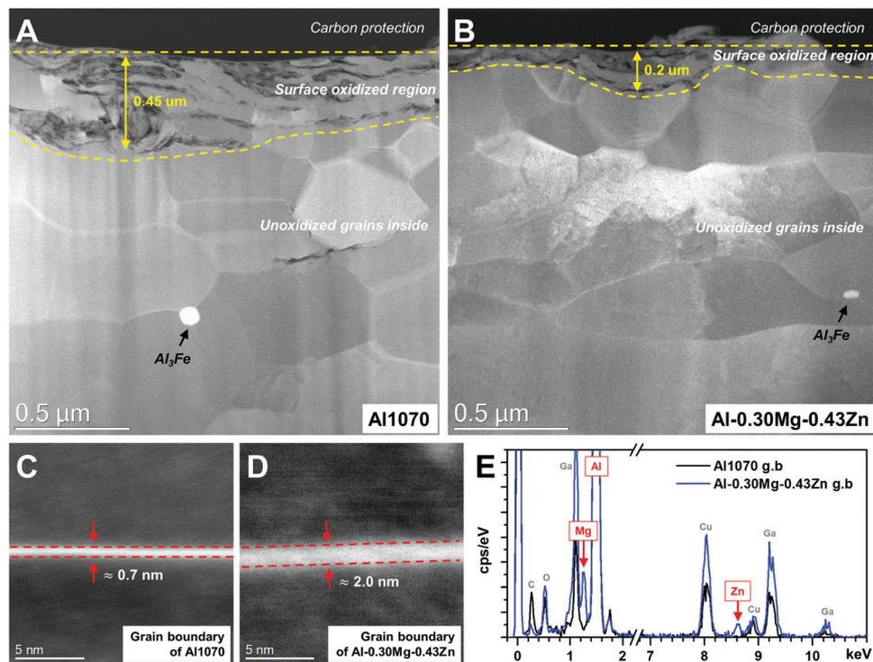
Fig. 5 Microstructures of Al1070 and Al-0.30Mg-0.43Zn. Low magnification STEM-HAADF images of (a) Al1070 and (b) Al-0.30Mg-0.43Zn. The grain boundaries of (c) Al1070 and (d) Al-0.30Mg-0.43Zn. (e) STEM-EDS analysis results at the grain boundary of Al1070 (black spectrum) and Al-0.30Mg-0.43Zn (blue spectrum).
