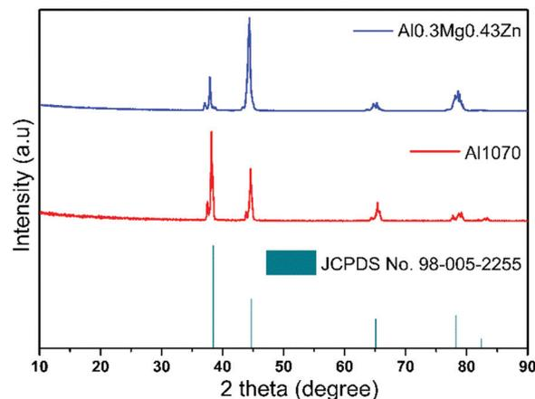
Fig. 6 X-Ray diffraction patterns of Al1070 and Al-0.30Mg-0.43Zn.
