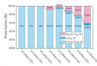
Fig. 2 Phase fraction calculation data of Al-xMg-yZn (0.10 < wt% of x <1.00, 0.10 < wt% of y < 0.55) samples.
