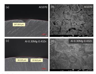
**Fig. 8** Optical microscope image showing the pitting depth of each sample after the 15 days SWAAT experiment: (a) Al 1070 and (c) Al-0.30Mg-0.43Zn. SEM image showing the surface of (b) Al 1070 and (d) Al-0.30Mg-0.43Zn.
