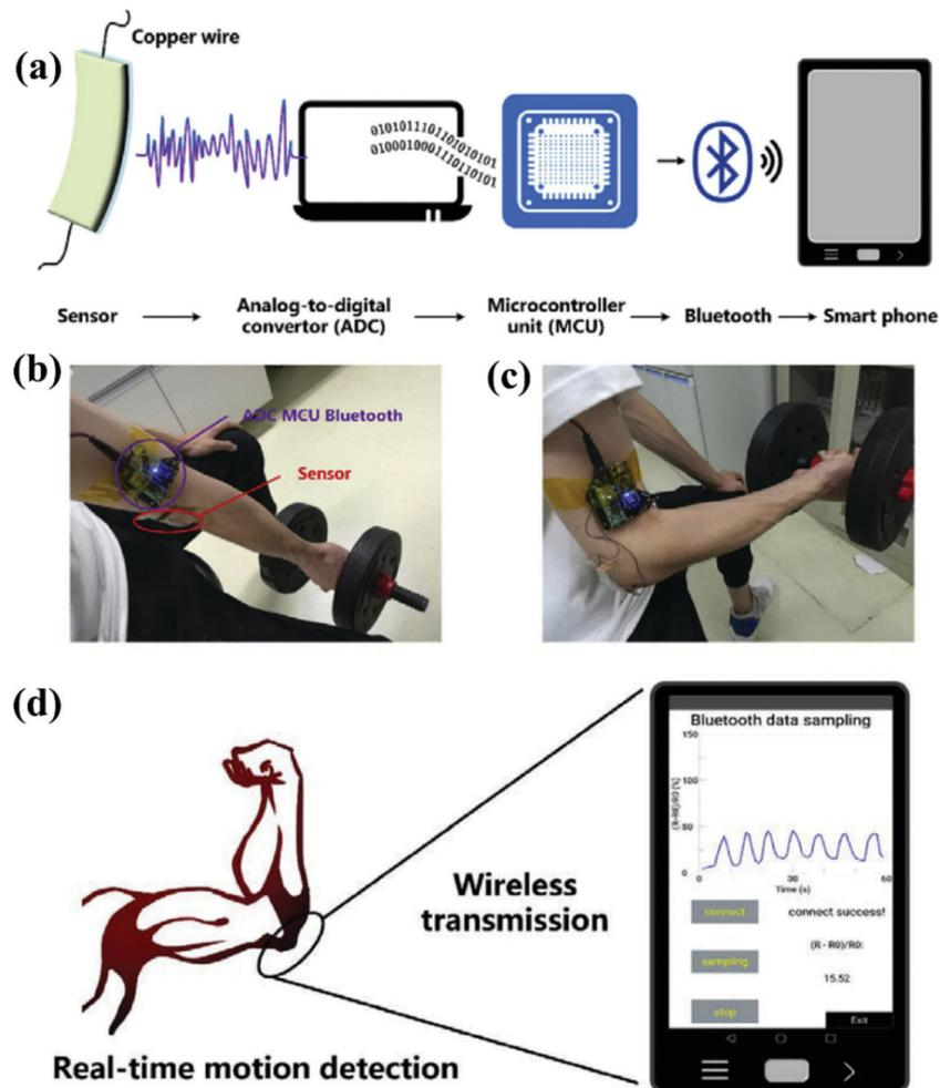
**Fig. 8** Real-time human machine interaction. (a) Schematic of a strain sensor based on a PAAm hydrogel system used to convert the digital signal through the ADC controlled by an MCU and then through wireless transfer of data to a smartphone using the bluetooth module. (b, c) The sensor mounted on an elbow to detect human motion like lifting of a dumbbell. (d) The interfacing of the app on a user's smart phone. Reproduced with permission from ref. 133.
