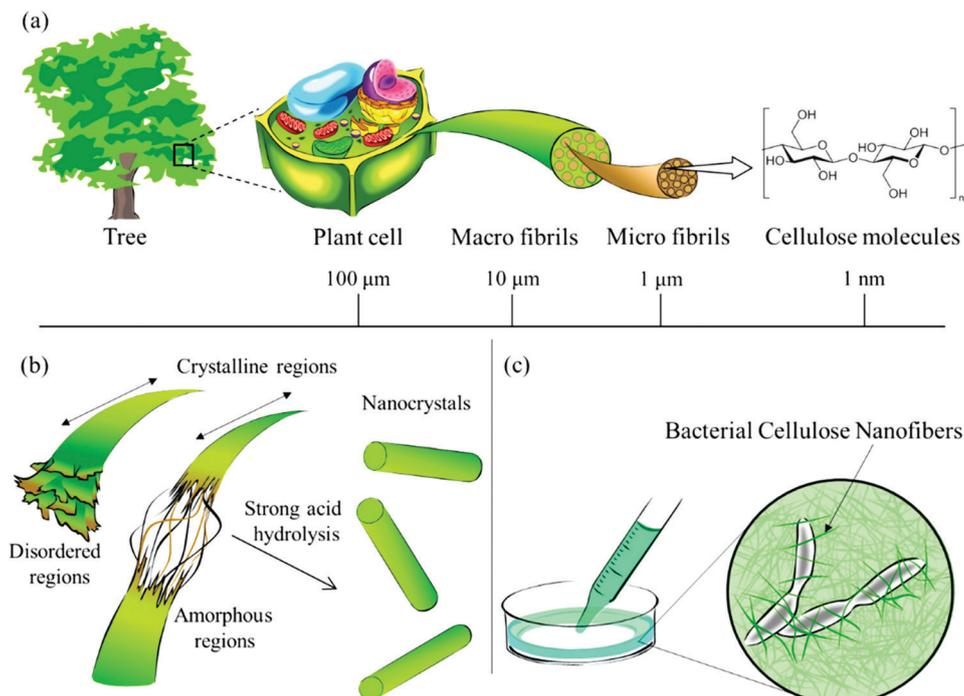
Fig. 2 (a) Cellulose derived from plants and its structure. (b) Hydrolysis reaction between the plant cellulose carried out to acquire nanocellulose. (c) Bacterial nanocellulose obtained using cellulose-synthesizing bacteria. Reproduced with permission from ref. 34.
