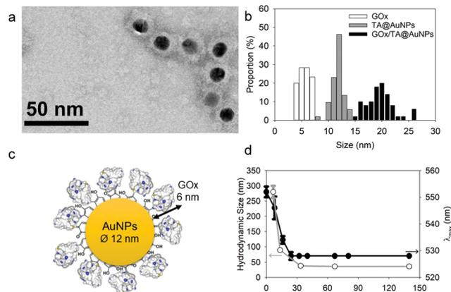
**Fig. 2** Characterization of GOx/TA@AuNPs complexes: (a) typical TEM image, obtained after uranyl acetate staining, (b) size distribution of GOx, TA@AuNPs and GOx/TA@AuNPs determined from TEM images with (c) the schematic illustration of GOx/TA@AuNPs (d) Aggregation test upon addition of 1 M NaCl in the GOx/TA@AuNPs suspension: the hydrodynamic size (white circle) and maximum absorption wavelength (black circle) values as a function of GOx/NPs molar ratio.
