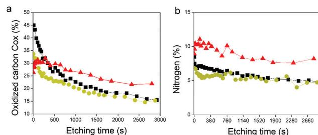
Fig. 8 Depth profiling of (a)  $C_{ox}$  and (b) nitrogen contributions the GOx/TA@AuNPs coating (red triangle), the GOx/TA@AuNPs drop-casted electrodeposition solution (yellow circle), and the GOx drop-casted solution (black square). The evolution is plotted as a function of the etching time by cluster argon bombardments at 8 keV and 300 atoms.
