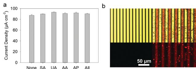
**Fig. 10** GOx/TA@AuNPs coating: (a) current density, measured at +0.25 V, of 5 mM glucose prepared in 0.5 mM FcOH/10 mM PBS in the absence (None) and the presence of different interfering substances, salicylic acid (SA), uric acid (UA), ascorbic acid (AA), acetaminophen (AP) and all of them (All) (b) Optical microscope images, in (top) bright field and (bottom) fluorescent mode, (left) before and (right) after electrodeposition of GOx<sup>Rho</sup>/TA@AuNPs coating.
