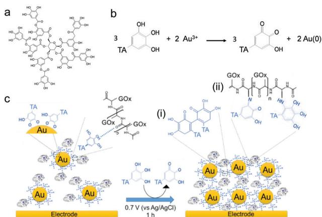
**Scheme 1** (a) Chemical formula of tannic acid (TA), (b) mechanism of TA@AuNPs synthesis by reduction of Au<sup>3+</sup> ions by TA in water. (c) Schematic representation of the electro-cross-linking of GOx/TA@AuNPs through electro-oxidation of gallol moieties of TA@AuNPs into quinone moieties followed by their chemical reaction with (i) gallol moieties of TA@AuNPs and (ii) free amino moieties of GOx through Michael addition and a Schiff's base condensation reaction.
