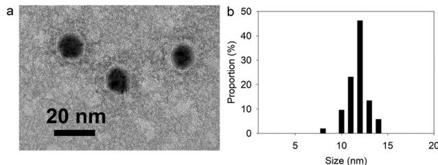
Fig. 1 Characterization of TA@AuNPs: (a) TEM image and (b) size distribution of TA@AuNPs determined from TEM images.
