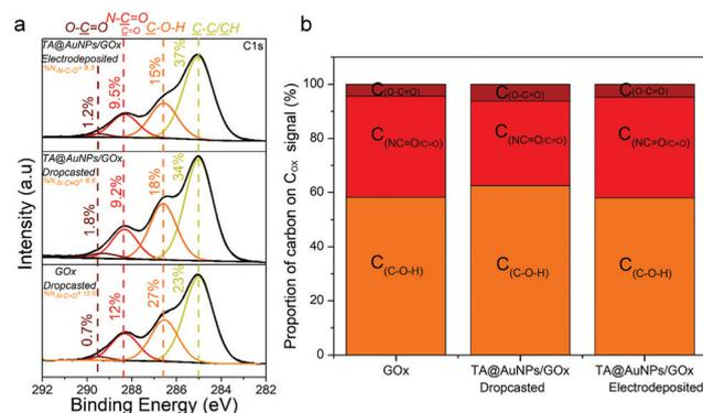
Fig. 7 (a) C 1s XPS spectra and (b) the relative contribution of each component in the oxidized organic carbon ( $C_{ox}$ ) signal of the GOx/TA@AuNPs coating, obtained by electrodeposition of FcOH/GOx/TA@AuNPs solution, the GOx/TA@AuNPs drop-casted electrodeposition solution and the GOx drop-casted solution.
