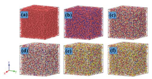
Fig. 1 Illustration of six FCC materials. (a-f) are Ni, FeNi, CrFeNi, CoCrFeNi, CoCrCuFeNi and CoCrFeMnNi, respectively
