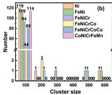
Fig. 2 (a) The number of defects in Ni, FeNi, CrFeNi, CoCrFeNi, CoCrCuFeNi and CoCrFeMnNi during the bombardment process. (b) The number of defect clusters in 0–100, 100–200, 200–300, 300–400, 400–500 and 500–600.
