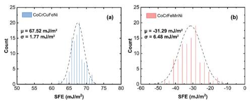
Fig. 6 The stacking fault energies of two kinds of high entropy alloys.  $\mu$  is the average fault energy of an alloy.  $\sigma$  is the standard deviation of the Gaussian curves, which are shown as dotted lines. (a) CoCrCuFeNi; (b) CoCrFeMnNi.
