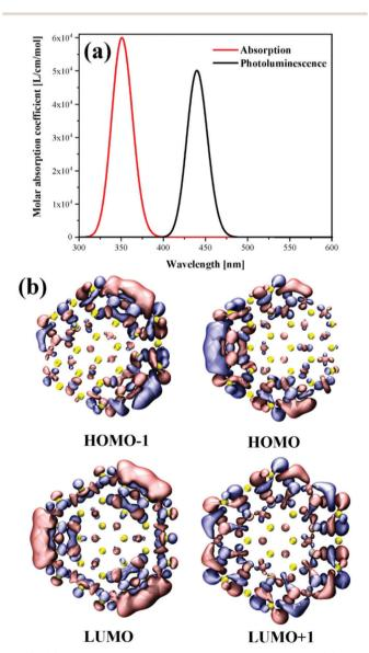
Fig. 10 (a) The calculated absorption and fluorescence spectra. (b) Frontier molecular orbitals of WS2 QDs.
