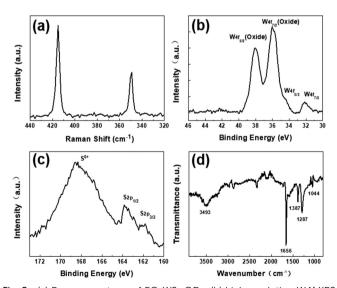
Fig. 8 (a) Raman spectrum of EG-WS $_2$  QDs; (b) high resolution W4f XPS spectrum of EG-WS $_2$  QDs; (c) High resolution S2p XPS spectrum of EG-WS $_2$  QDs; (d) EG-Fourier infrared spectrum of WS $_2$  QDs.
