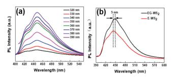
Fig. 9 (a) Photoluminescence spectra of EG-WS<sub>2</sub> QDs with excitation from 320 nm to 390 nm; (b) Fluorescence spectra of EG-WS2 QDs and ethanol passivated WS2 QDs (E-WS2 QDs).
