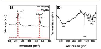
Fig. 4 (a) Comparison of Raman spectra of bulk  $WS_2$  and  $WS_2$  QDs; (b) Fourier infrared spectra of  $WS_2$  QDs.
