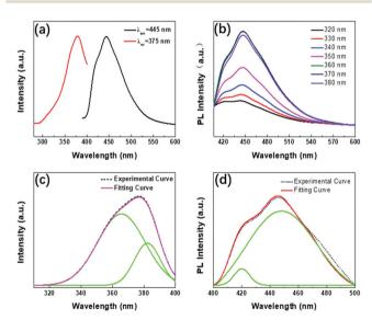
Fig. 5 (a) Absorption and photoluminescence spectra of WS<sub>2</sub> QDs dispersed in ethanol solvent; (b) photoluminescence spectra of WS<sub>2</sub> QDs with increasing excitation wavelength; (c) monitoring at 445 nm Fluorescence emission peak, get the photoluminescence excitation spectrum of WS<sub>2</sub> QDs (dotted line) and the fitted Lorentz spectrum; (d) the photoluminescence excitation spectrum of WS2 QDs (dotted line) and the fitted Lorentz
