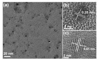
Fig. 1 (a) TEM image of WS<sub>2</sub> QDs; (b and c) HRTEM images of WS<sub>2</sub> QDs
