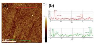
Fig. 2 (a) AFM diagram of WS $_2$  QDs; (b) height distribution statistics curve of WS $_2$  QDs along the red and green lines in (a).
