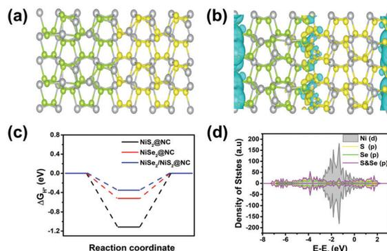
Fig. 7 (a) The theoretical models of NiSe<sub>2</sub>/NiS<sub>2</sub>@NC used in the DFT calculations. (b) Differential charge density between NiS<sub>2</sub>@NC and NiSe<sub>2</sub>@NC. (c) The projected electronic density of states (PDOS) of NiSe<sub>2</sub>/NiS<sub>2</sub>@NC. (d) Gibbs free-energy diagram for H\* adsorption ( $\Delta G_{H^*}$ ).
