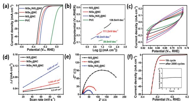
Fig. 6 The HER performance in 1.0 M KOH solution: (a) LSV curves; (b) Tafel plots; (c) the CV curves of NiSe<sub>2</sub>/NiS<sub>2</sub>@NC; (d) the  $C_{dl}$ ; (e) EIS data; (f) LSV curves of NiSe<sub>2</sub>/NiS<sub>2</sub>@NC before and after 2000 cycles of the stability test. (Inset: time dependent current density ( $i-t$ ) curves of NiSe<sub>2</sub>/NiS<sub>2</sub>@NC).
