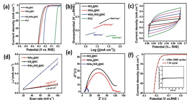
Fig. 5 The HER performance in 0.5 M  $\text{H}_2\text{SO}_4$  solution: (a) LSV curves; (b) Tafel plots; (c) the CV curves of  $\text{NiSe}_2/\text{NiS}_2@\text{NC}$ ; (d) the electrochemical double-layer capacitance ( $C_{dl}$ ); (e) EIS data; (f) LSV curves of  $\text{NiSe}_2/\text{NiS}_2@\text{NC}$  before and after 2000 cycles for stability test. (Inset: time dependent current density ( $i-t$ ) curves of  $\text{NiSe}_2/\text{NiS}_2@\text{NC}$ ).
