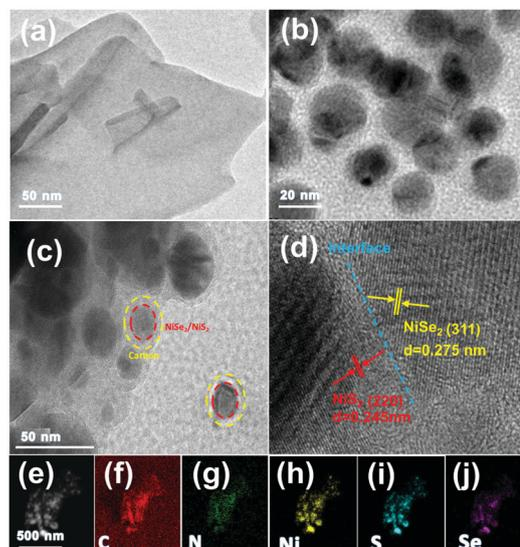
Fig. 3 (a) TEM image of the MOF. (b) TEM image of the Ni@NC. (c) TEM image of the NiSe<sub>2</sub>/NiS<sub>2</sub>@NC. (d) HRTEM image of the NiSe<sub>2</sub>/NiS<sub>2</sub>@NC. (e–j) EDS elemental mapping images showing C, N, Ni, S, and Se in the NiSe<sub>2</sub>/NiS<sub>2</sub>@NC.
