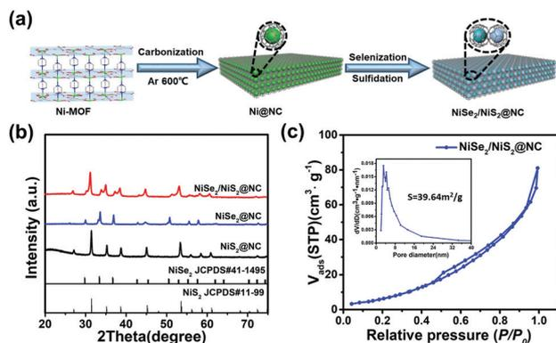
Fig. 1 (a) Schematic illustration of the two-step synthetic procedures of NiSe<sub>2</sub>/NiS<sub>2</sub>@NC. (b) XRD patterns. (c) N<sub>2</sub> adsorption-desorption isotherms (inset: pore size distribution curve).
