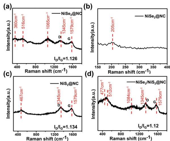
Fig. 2 Raman spectra of (a) and (b) NiSe<sub>2</sub>@NC, (c) NiS<sub>2</sub>@NC, and (d) NiSe<sub>2</sub>/NiS<sub>2</sub>@NC.
