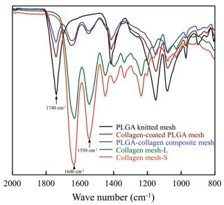
Fig. 2 ATR-FTIR spectra of PLGA mesh, collagen-coated PLGA mesh, PLGA-collagen composite mesh, collagen mesh-L and collagen mesh-S in the absorption band from 2000 to 800 cm<sup>-1</sup>.
