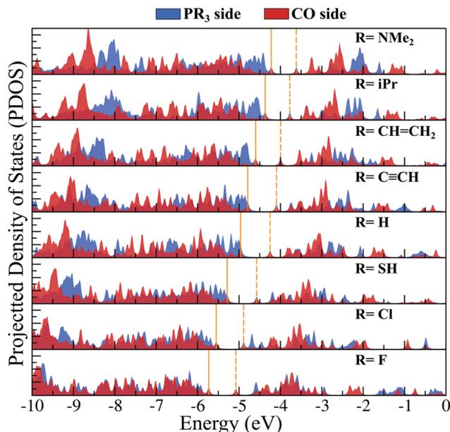
Fig. 8 The projected density of state (PDOS) diagram of  $(\text{PR}_3)_5\text{Rh}_6\text{S}_8\text{-Rh}_6\text{S}_8(\text{CO})_5$  ( $\text{R} = \text{NMe}_2$  to  $\text{F}$ ) dimers. The location of the HOMO and LUMO levels are marked by solid and dashed lines, respectively. The contributions from  $\text{PR}_3$  and  $\text{CO}$  side are shown in blue and red color, respectively.
