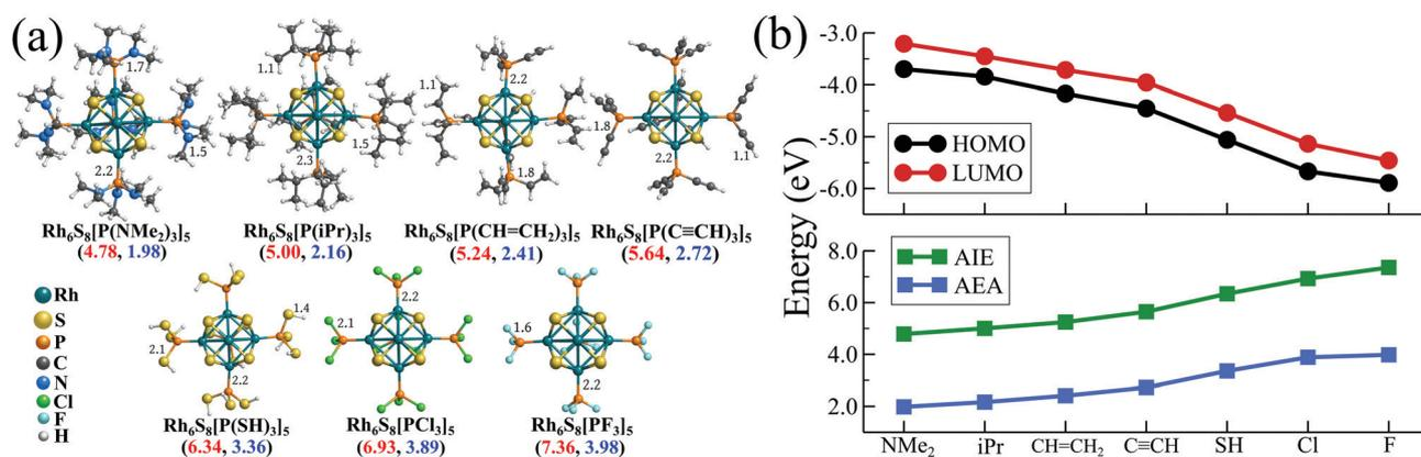
Fig. 2 (a) The optimized ground state structures of  $\text{Rh}_6\text{S}_8(\text{PR}_3)_5$  (R = NMe<sub>2</sub> to F). Bond lengths are in Å. The AIE (red) and AEA (blue) values (in eV) are included within parenthesis. (b) The plot of HOMO–LUMO gap, AIE and AEA of  $\text{Rh}_6\text{S}_8(\text{PR}_3)_5$  clusters.
