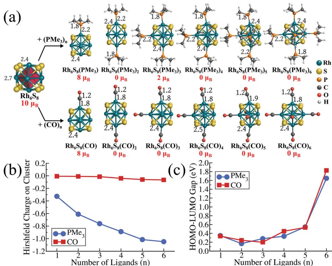
Fig. 1 (a) The optimized ground state structures and magnetic moments of  $\text{Rh}_6\text{S}_8$  and  $\text{Rh}_6\text{S}_8\text{L}_n$  ( $\text{L} = \text{PMe}_3$ ,  $\text{CO}$ ;  $n = 1-6$ ) clusters. Bond lengths are in Å. (b) The variation of Hirshfeld charge and HOMO–LUMO gap along the  $\text{Rh}_6\text{S}_8\text{L}_n$  series.
