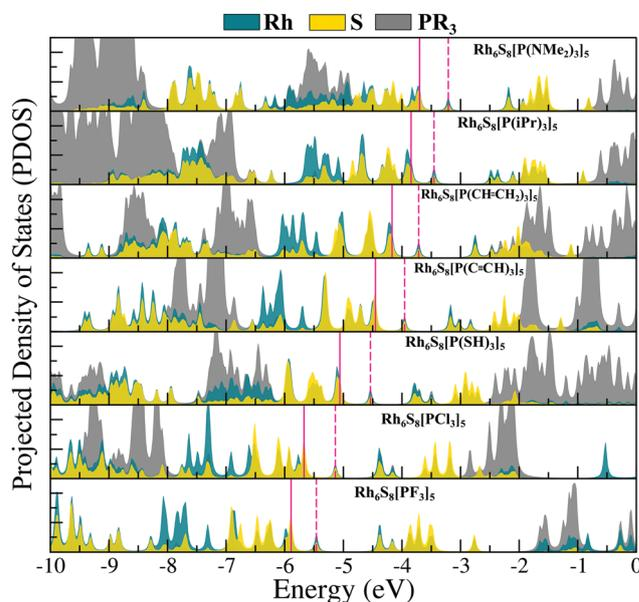
Fig. 4 The projected density of state (PDOS) diagram of  $\text{Rh}_6\text{S}_8(\text{PR}_3)_5$ , ( $\text{R} = \text{NMe}_2$  to  $\text{F}$ ) clusters. The location of the HOMO and LUMO levels are marked by solid and dashed lines, respectively. The contributions from Rh, S and the  $\text{PR}_3$  ligands are shown in different colors.
