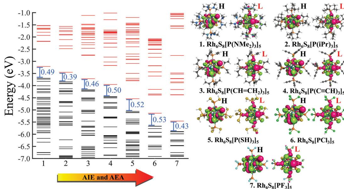
Fig. 3 The molecular orbital (MO) diagram of  $\text{Rh}_6\text{S}_8(\text{PR}_3)_5$ , ( $\text{R} = \text{NMe}_2$  to  $\text{F}$ ) clusters. The black and red lines show the occupied and unoccupied MOs, respectively. The HOMO (H) and LUMO (L) isosurfaces for all ligated clusters are shown on right.
