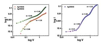
Fig. 10 Log / vs. log V plot of Ag/10S/Si, Ag/30S/Si and Ag/20S/Si diode. m is the slope of the curve.
