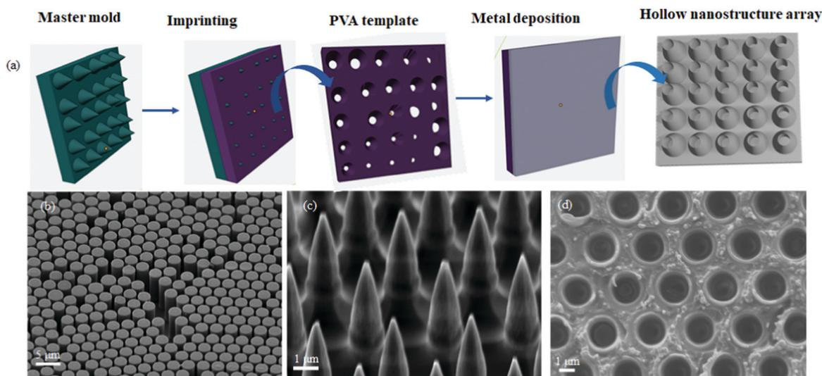
**Fig. 1** (a) Illustration of the preparation of hollow metal nanostructures. Surface morphology of (b) Si micropillars formed through the Bosch process for 24 cycles, (c) Si master mould formed after pseudo etching the Si micropillars for 3.15 min, (d) PVA template.
