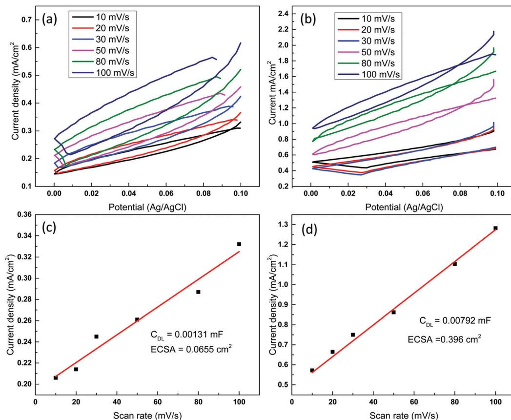
Fig. 4 Cyclic voltammetry recorded at various scanning rate in the presence of  $0.5 \text{ M KHCO}_3$  over (a) plain copper film, (b) Cu hollow nanostructures. Plots for current vs. scan rate for (c) plain copper film, (d) copper hollow nanostructure. The slope for the plots provided double layer capacitance ( $C_{\text{DL}}$ ) values.
