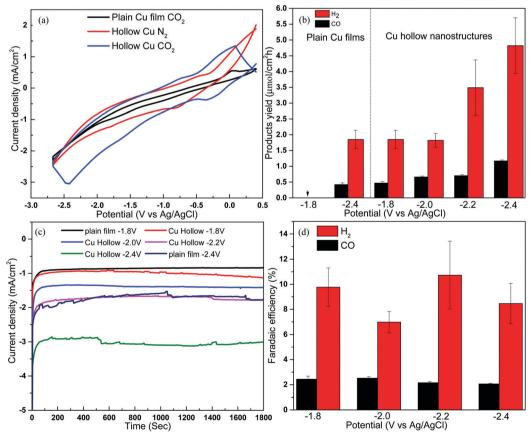
Fig. 3 (a) Cyclic voltammetry at a scanning rate of 50 mV s<sup>-1</sup>, (b) products yield for electrocatalytic conversion of  $CO_2$  in the presence of 150 mM [C<sub>2</sub>mimOAc] dissolved in DMAC (c) current density, (d) faradaic efficiency for the Cu hollow nanostructures.
