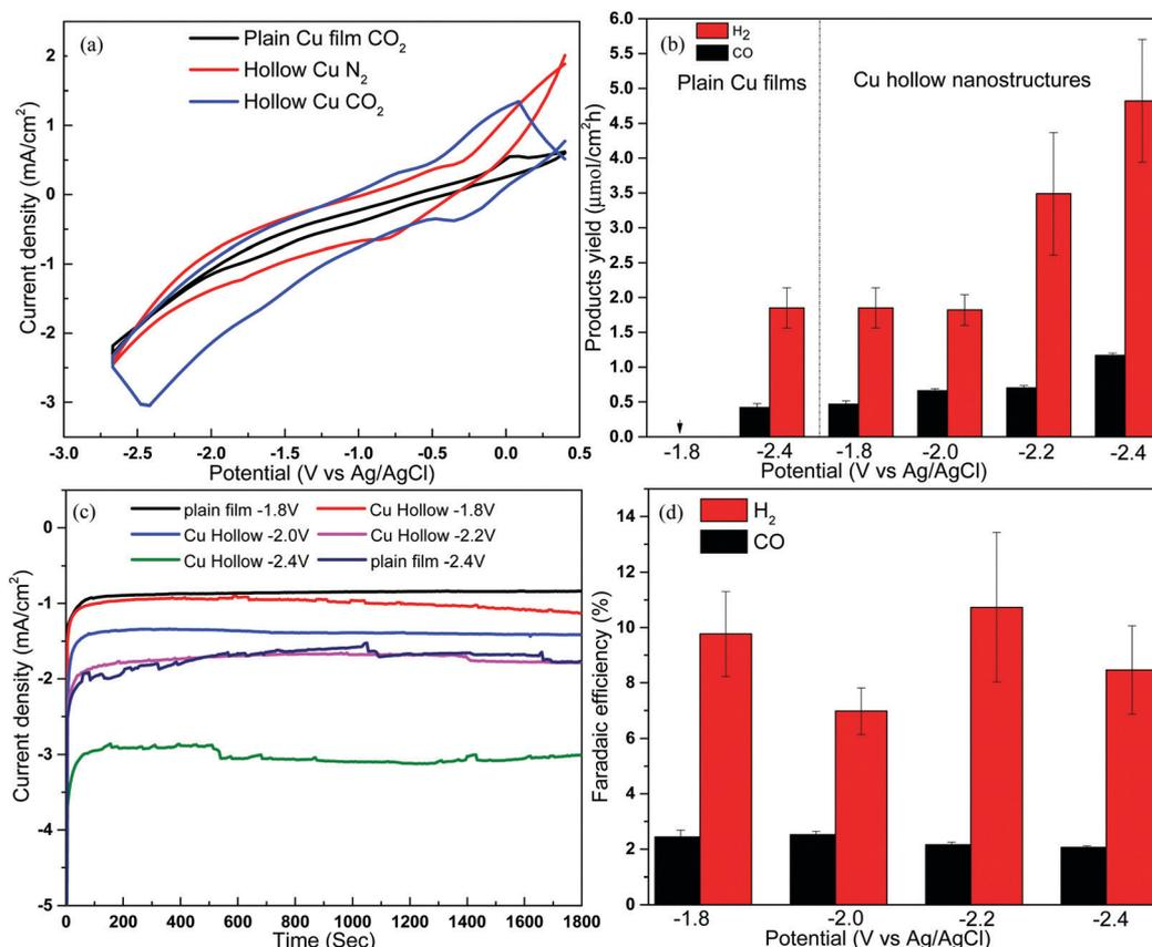
Fig. 3 (a) Cyclic voltammetry at a scanning rate of  $50 \text{ mV s}^{-1}$ , (b) products yield for electrocatalytic conversion of  $\text{CO}_2$  in the presence of 150 mM  $[\text{C}_2\text{mimOAc}]$  dissolved in DMAC (c) current density, (d) faradaic efficiency for the Cu hollow nanostructures.
