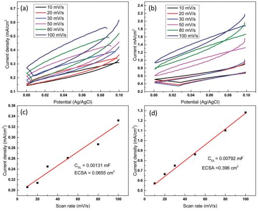
Fig. 4 Cyclic voltammetry recorded at various scanning rate in the presence of 0.5 M KHCO<sub>3</sub> over (a) plain copper film, (b) Cu hollow nanostructures. Plots for current vs. scan rate for (c) plain copper film, (d) copper hollow nanostructure. The slope for the plots provided double layer capacitance ( $C_{DL}$ ) values.
