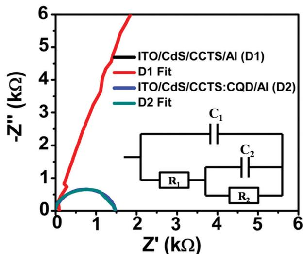
Fig. 11 Nyquist plots of the impedance data of the CCTS and CCTS:CQD heterojunction films in the dark.
