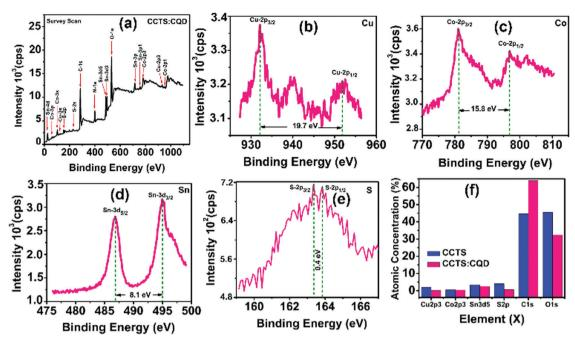
Fig. 3 XPS analysis of CCTS:CQD thin film: (a) survey spectrum with corresponding elements of (b) Cu 2p, (c) Co 2p, (d) Sn 3d and (e) S 2p. (f) Atomic percentages of CCTS and CCTS:CQD thin films
