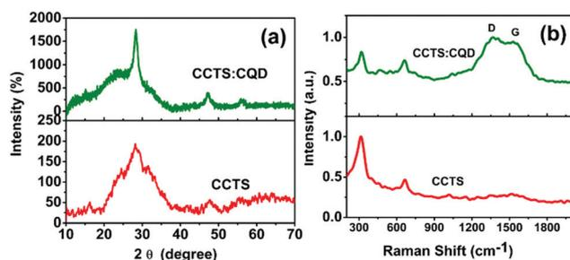
Fig. 1 (a) XRD patterns and (b) Raman spectra of CCTS and CCTS:CQD thin films.
