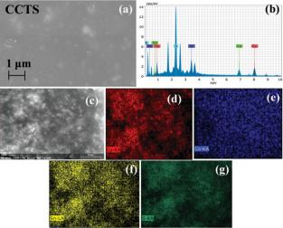
Fig. 5 (a) FESEM image of CCTS. (b) EDS spectrum and elemental mapping of CCTS as (c) morphology at 5  $\mu m$  for mapping (d) Cu, (e) Co, (f) Sn and (g) S.
