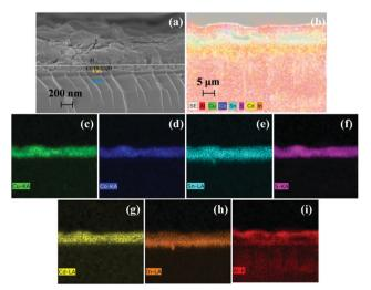
Fig. 7 (a) Cross-sectional FESEM image of ITO/CdS/CCTS:CQD/Al device. (b) Cross section in 5 µm scale for elemental mapping. The elemental distributions of (c) Cu, (d) Co, (e) Sn, (f) S, (g) Cd, (h) In and (i) Al.
