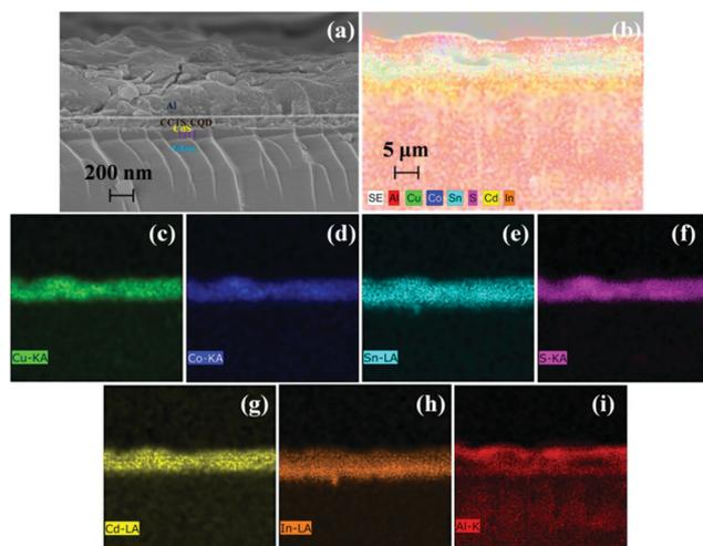
Fig. 7 (a) Cross-sectional FESEM image of ITO/CdS/CCTS:CQD/Al device. (b) Cross section in 5  $\mu\text{m}$  scale for elemental mapping. The elemental distributions of (c) Cu, (d) Co, (e) Sn, (f) S, (g) Cd, (h) In and (i) Al.
