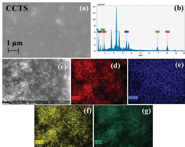
Fig. 5 (a) FESEM image of CCTS. (b) EDS spectrum and elemental mapping of CCTS as (c) morphology at 5  $\mu\text{m}$  for mapping (d) Cu, (e) Co, (f) Sn and (g) S.
