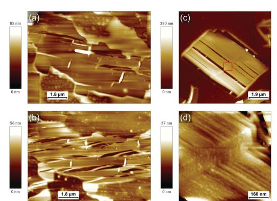
Fig. 4 AFM images of the same crystal of PDA (a) before and (b) after heating at 75 °C for 2 h. (c and d) AFM image of another PDA crystal after annealing at 95  $^{\circ}\text{C}$  for 5 min. The AFM image in (d) correspond to the red rectangle in (c).
