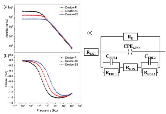
Fig. 2 ElS curves of  $Ru(bpy)_3(PF_6)_2$  memristor devices with different concentrations of  $LiClO_4$ . (a) Impedance *versus* frequency data and (b) phase *versus* frequency data for Device-P (black squares), Device-1S (red circles), and Device-2S (blue triangles). (c) An equivalent circuit employed for ElS fitting of the OMIEC memristor devices.
