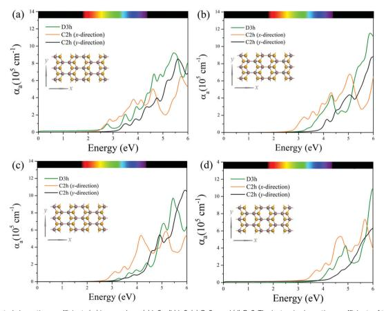
Fig. 5 Calculated absorption coefficients ( $\alpha_a$ ) in monolayer (a) InSe, (b) InS, (c) GaSe, and (d) GaS. The isotropic absorption coefficients of the  $D_{3h}$  phases are shown in green. For the  $C_{2h}$  monolayers, the absorption coefficients along the x-direction are shown in orange and those along the y-direction are shown in black. The insets show the two in-plane directions with respect to the top view of the  $C_{2h}$  structure.
