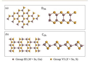
Fig. 1 The monolayer structures of (a)  $D_{3h}$  and (b)  $C_{2h}$  MXs. The top and side views are presented on the left and the right side of each panel respectively. The structural coordinates of  $C_{2h}$  monolayers can be found in
