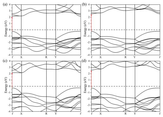
Fig. 3 Computed electronic band structures of monolayer  $C_{2h}$  (a) InSe, (b) InS, (c) GaSe, and (d) GaS at the HSE06 level. The red arrows point from VBM to CBM (direct band gaps at the  $\Gamma$  points). The values of the band gaps can be found in Table S1 (ESI†).
