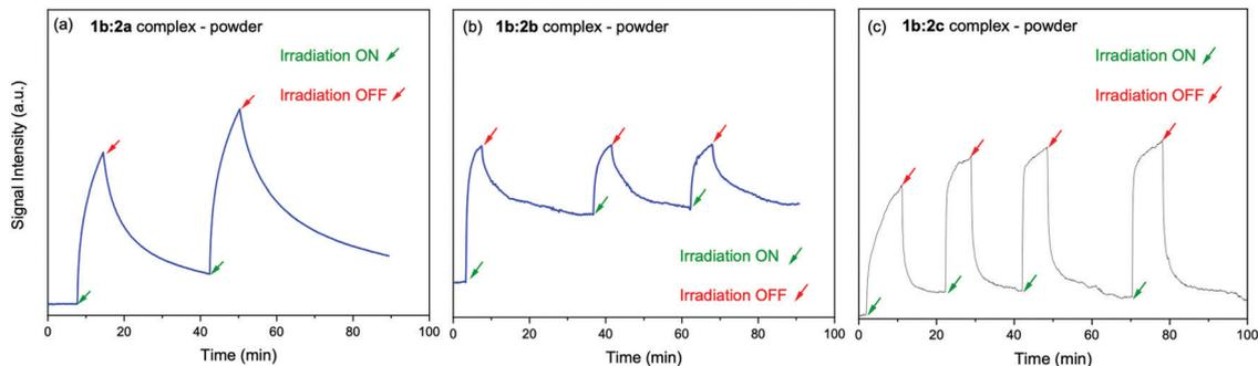
Fig. 9 Time evolution of the EPR signal at 346 mT recorded in the presence and absence of light irradiation at 410 nm. Powder samples: (a) **1b:2a**, (b) **1b:2b**, (c) **1b:2c** complexes.
