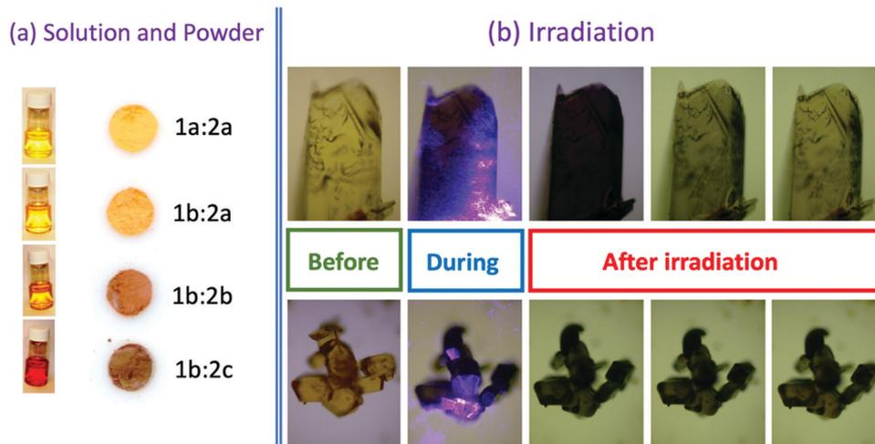
Fig. 1 (a) Four charge-transfer complexes with different coloration in saturated solution and solid phase (powder). (b) Photochromic changes of the **1b:2b** (top side) and **1b:2c** (bottom side) complexes during and after irradiation at 410 nm;  $T = 298$  K.
