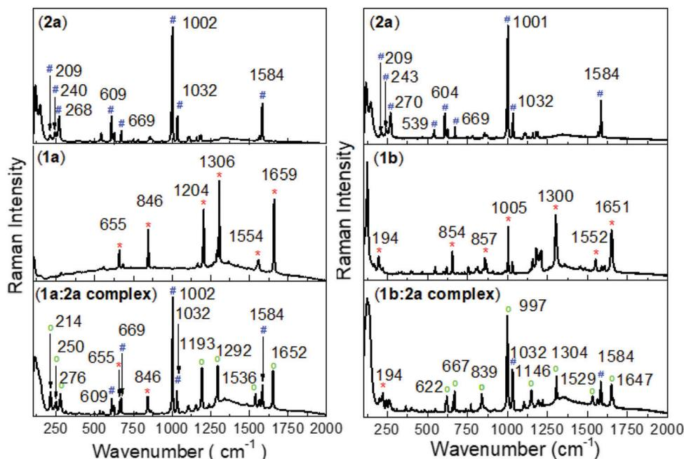
Fig. 3 Raman spectra of the precursor salts and their complex forms. (2a) potassium tetraphenylborate; (1a) methyl viologen dichloride; (1b) benzylviologen dichloride.  $\lambda_{\text{laser}} = 780$  nm. Characteristic Raman features of (#) potassium tetraarylborate, (\*) viologen dichloride and (O) the ion pair complex.
