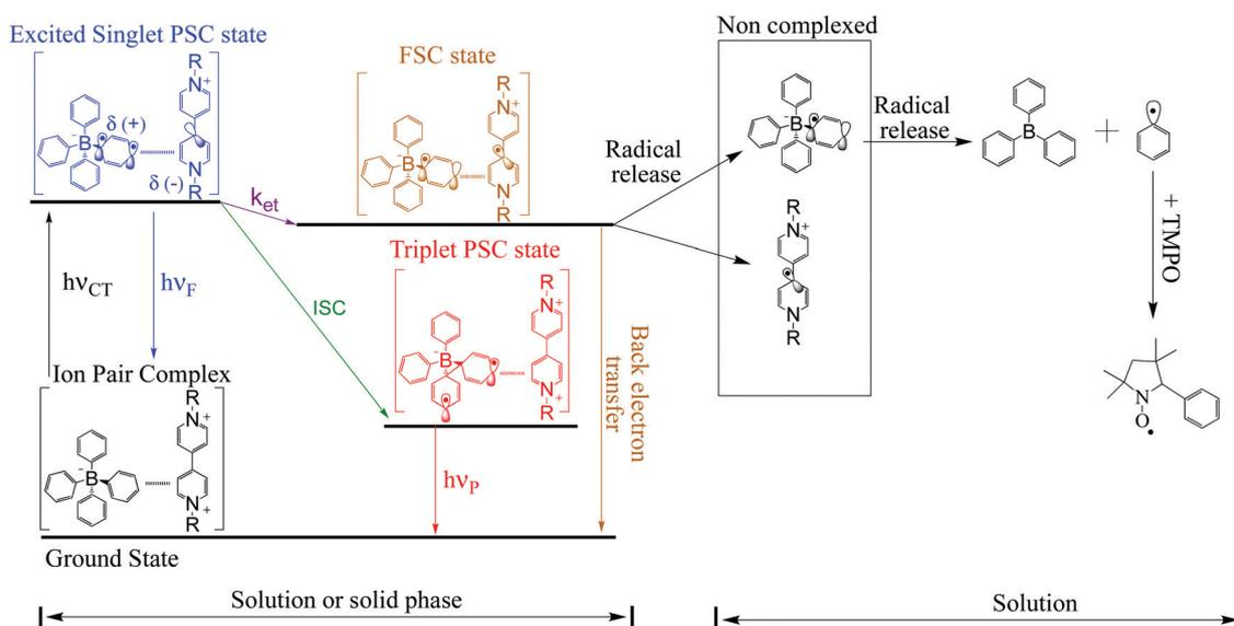
Scheme 3 Schematic diagram for FSC-state and PCS-state deactivation.
