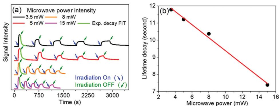
Fig. 8 (a) Time evolution of the EPR signal at 346 mT recorded at different microwave power intensity. Sample: **1a:2a** complex in solid phase (powder). (b) Direct correlation between microwave power and lifetime decay.
