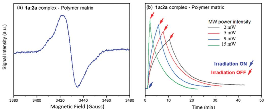
Fig. 11 (a) SSEPR spectrum of the **1a:2a** complex in thin film of PEVA. (b) Time profiles of the SSEPR signal of the viologen radical at different  $\mu\text{W}$  powers (in mW) in the polymer matrix, in the presence and absence of light irradiation at 410 nm.
