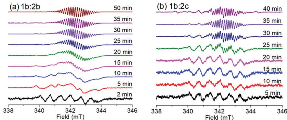
Fig. 6 Time evolution of the maximum EPR signal of (a) **1b:2b** complex and (b) **1b:2c** complex recorded at different times of irradiation in THF : ACN (5 : 1 v/v) solvent, [complex] =  $10^{-3}$  mol L $^{-1}$ ;  $\lambda_{irr}$  = 410 nm.
