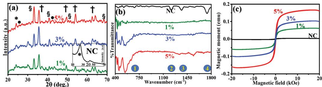
Fig. 5 (a) XRD spectra recorded in the  $2\theta$  range of  $20\text{--}70^\circ$  displaying the diffraction peaks indicated by various symbols (inset: NC plot), (b) recorded FTIR spectra in the range of  $400\text{--}1800\text{ cm}^{-1}$ , exhibiting the typical functional groups (1–4), where data is shown for NC and FNC (1%, 3%, and 5%)-composites, and (c) measured vibrating sample magnetometry profiles for the NC and FNC samples (typically displayed for 1%, 3%, and 5%) at 300 K.
