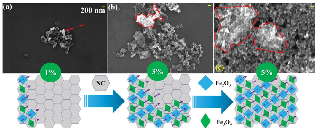
Fig. 6 SEM micrographs recorded for 1%, 3%, and 5% FNC composite at 30 $\times$  magnification (scale bar: 200 nm). Red dotted line contour displays coverage of Fe/Fe<sub>3</sub>O<sub>4</sub>/Fe<sub>2</sub>O<sub>3</sub> on the NC network. Panel below shows the coverage scheme.
