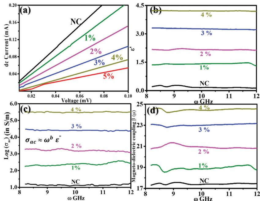
Fig. 9 (a)  $I$ - $V$  profiles recorded, (b) estimated  $\epsilon'$ , (c) calculated ac conductivity,  $\sigma_{ac}$  (in log-normal scale), and (d) estimated magneto-dielectric coupling,  $\beta$  ( $\mu$ ), for the NC and FNC composite over the 8–12 GHz (X-band) regime.
