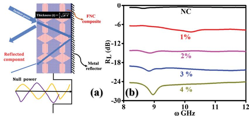
Fig. 12 (a) Sketch of the Dallenbach scattering technique for the reflection loss ( $R_L$ ) analysis of the NC/FNC coatings. Condition on thickness in terms of constitutive parameters is displayed on the top for the composite layers, attached metal support, schematic of power losses from first and second interface, and null/minimum power condition at the bottom. (b) Recorded  $R_L$  spectra for NC and (1–4%) FNC-composites over 8–12 GHz.
