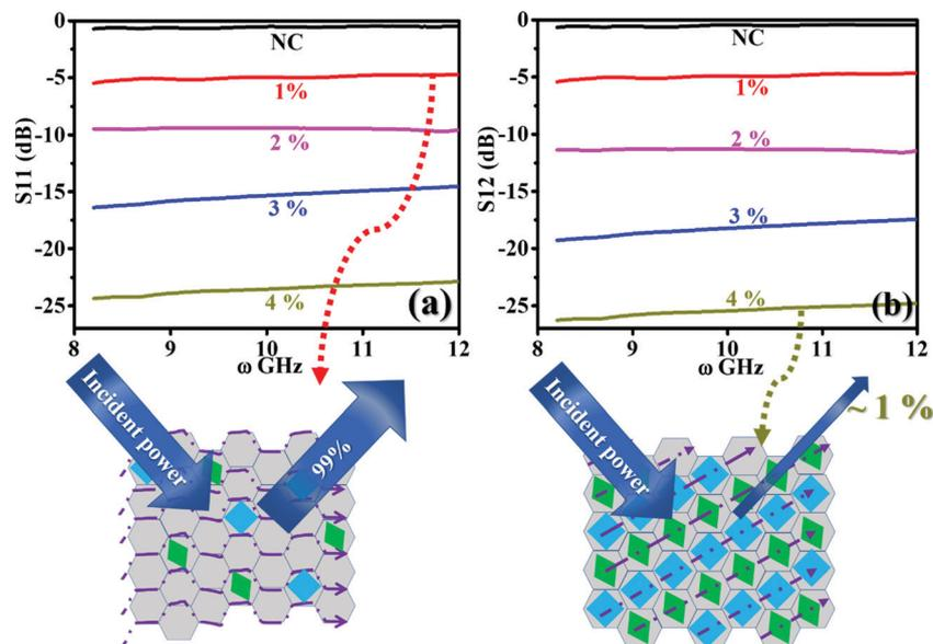
Fig. 11 Port  $S$ -parameter behaviour recorded at (a)  $S_{11}$  and (b)  $S_{12}$  interface of NC and 1–4% FNC-composites in the X-band regime. Scheme below plot (a) shows  $\sim 80\%$  reflection at 1% FNC, whereas the scheme below plot (b) shows almost  $\sim 99\%$  reduction in reflection at 4% FNC composition. The shielding effectiveness data is tabulated in Table 3.
