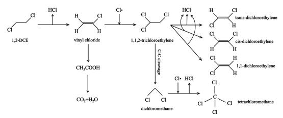
Scheme 1 The possible mechanisms of 1,2-DCE catalyst combustion over MnO<sub>2</sub>.
