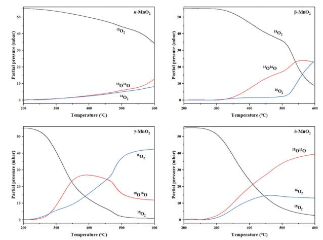
Fig. 6 Temperature programmed reaction of the  ${}^{18}\text{O}_2/{}^{16}\text{O}_2$  isotopic exchange of MnO<sub>2</sub>.
