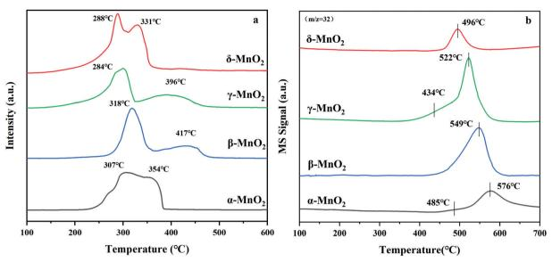
Fig. 4 The (a) H<sub>2</sub>-TPR and (b) O<sub>2</sub>-TPD profiles of MnO<sub>2</sub>.
