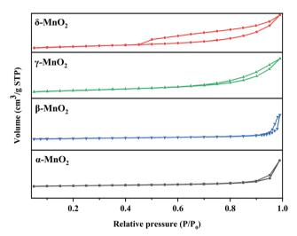
Fig. 2 The nitrogen adsorption-desorption isotherms of MnO<sub>2</sub>.
