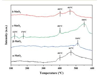
Fig. 8 The NH<sub>3</sub>-TPD profile of MnO<sub>2</sub>.
