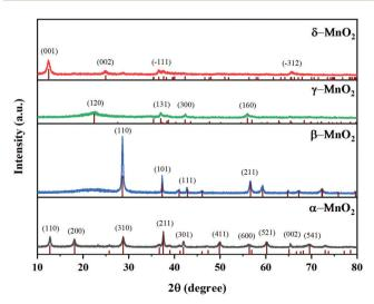
Fig. 1 The XRD patterns of MnO<sub>2</sub>
