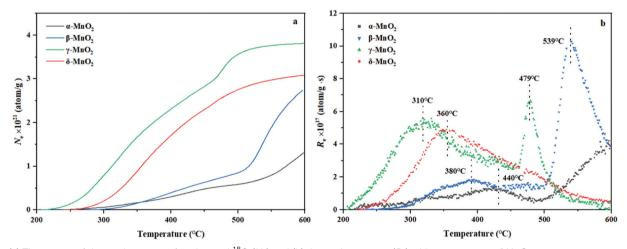
Fig. 7 (a) The curves of the total amount of exchanged  $^{18}$ O ( $N_{\rm e}$ ) and (b) the exchange rate ( $R_{\rm e}$ ) with temperature of MnO<sub>2</sub>.
