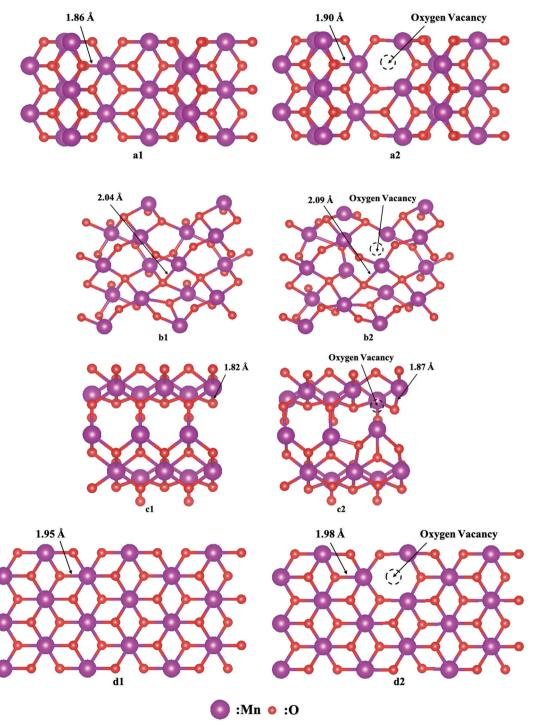
Fig. 11 Model structures of (a)  $\alpha$ -, (b)  $\beta$ -, (c)  $\gamma$ - and (d)  $\delta$ -MnO<sub>2</sub> (a1-d1) without and (a2-d2) with oxygen vacancies.
