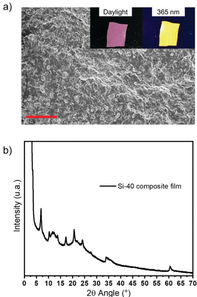
Fig. 10 (a) SEM image (scale bar = 20  $\mu\text{m}$ ); inset: photographs of the Si-40 composite film under daylight and under UV light at 365 nm and (b) X-ray diffraction pattern of the Si-40 composite film.
