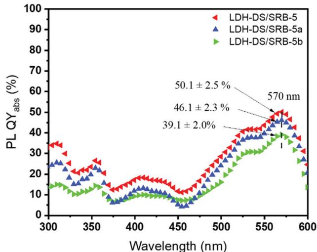
Fig. 6 Absolute PLQY in the 360–600 nm excitation wavelength range for samples LDH-DS/SRB-5, 5a and 5b.
