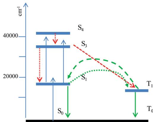
**Fig. 12** Proposed de-excitation mechanism of SRB in the LDH–DS/SRB-5 powder.
