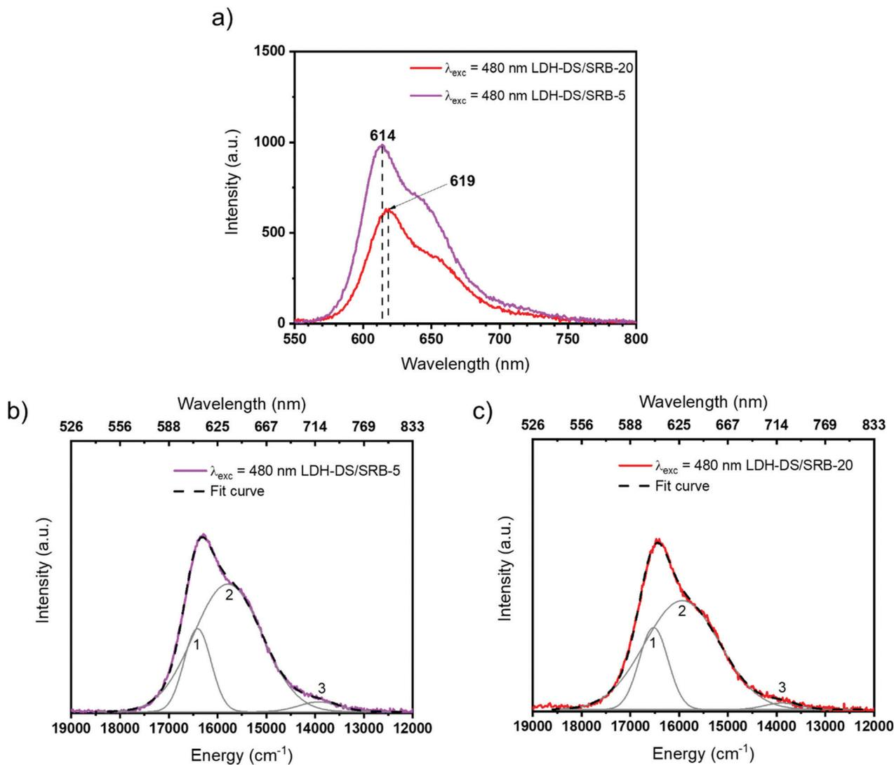
Fig. 3 (a) Emission spectra of LDH-DS/SRB-5 and -20 ( $x = 0.0005$  and  $0.002$ , respectively) powders under excitation at  $480$  nm; (b) and (c) Gaussian-type deconvolution for LDH-DS/SRB-5 and -20 emission bands, respectively.
