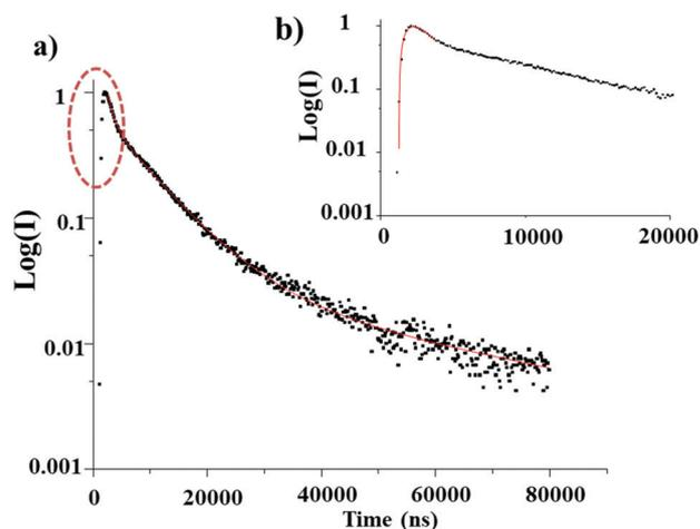
Fig. 11 (a) Luminescence decay of the LDH–DS/SRB-5 powder ( $\lambda_{\text{exc}} = 400$  nm and  $\lambda_{\text{em}} = 604$  nm); experimental curve in dots and the fit in red solid line; equation used for the fit:  $y = A_1 \times \exp(-x/\tau_1) + A_2 \times \exp(-x/\tau_2) + A_3 \times \exp(-x/\tau_3)$ , (b) rise time fitting:  $(y = -A_1 \times \exp(-x/\tau_4) + A_2 \times \exp(-x/\tau_1))$ .
