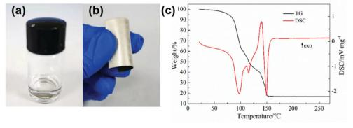
Fig. 1 (a) Image of silver oxalate-1,2-diaminopropane ink, (b) image of the silver film, and (c) the TG-DSC curve of the ink.
