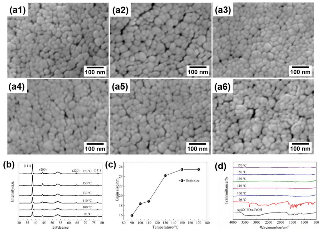
Fig. 2 Characterization of films thermally treated at different temperatures. (a1–a6) SEM images. (a1) 90 °C, (a2) 100 °C, (a3) 110 °C, (a4) 130 °C, (a5) 150 °C, and (a6) 170 °C. (b) XRD patterns, (c) grain size and (d) FTIR spectrum.
