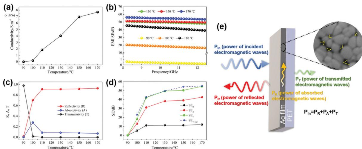
Fig. 3 Properties of silver films thermally treated at different temperatures, (a) conductivities, (b) EMI SE in the X band, (c) power coefficients  $R$ ,  $A$ , and  $T$ , (d) the comparison of  $SE_R$ ,  $SE_A$ ,  $SE_T$ , and  $SE_{T\_Cal}$  at 10.3 GHz, and (e) schematic EMI shielding mechanism of the nanoparticle silver film.
