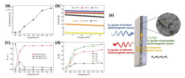
Fig. 3 Properties of silver films thermally treated at different temperatures, (a) conductivities, (b) EMI SE in the X band, (c) power coefficients R, A, and T, (d) the comparison of SE $_R$ , SE $_R$ , SE $_T$ , and SE $_T$ Cal at 10.3 GHz, and (e) schematic EMI shielding mechanism of the nanoparticle silver film.
