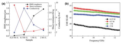
Fig. 5 (a) RMS roughness, sheet resistance and conductivity of films with different concentrations. (b) EMI SE in the X band
